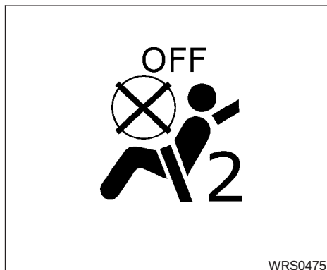
Front passenger air bag and status light
