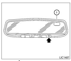
Press the - 1 button for about 1 second when the ignition switch is placed in the ON position to toggle the compass display 1 on or off. The display will indicate the direction of the vehicle's heading.
