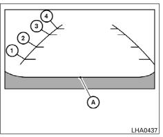
They are indicated as reference distances to objects. The lines and colors in the display indicate distances from the back bumper line (A) in the illustration.
