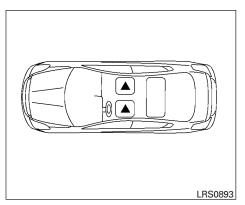
The illustration shows the seating positions equipped with head restraints. All of the head restraints are adjustable.
