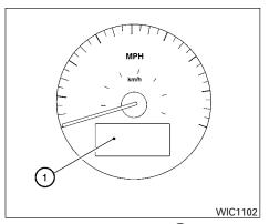
The vehicle information display (1) is located on the bottom of the speedometer. It displays such items as:
