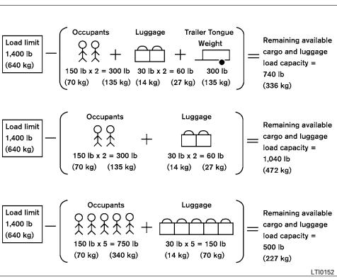
Steps for determining correct load limit
