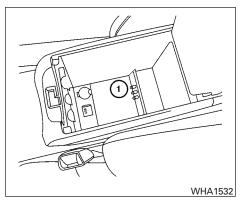
Before connecting a device to the auxiliary input iacks, turn off the power of the portable device.
