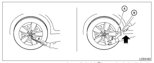
Removing the bolt-on wheel cover (if so equipped)
