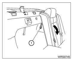
To fold down the driver's side of the rear seat. reach through the opening and pull on the strap (1) located behind the seat.
