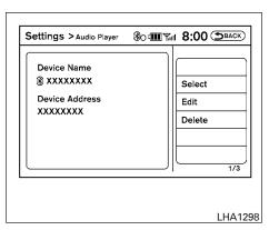
6. The Device Name and Device Address are displayed on the screen. Select the "Select" key to make this device the active Bluetooth® audio player. Select the "Edit" key to edit the details of the player, such as Device Name. Select the "Delete" key to delete the device.
