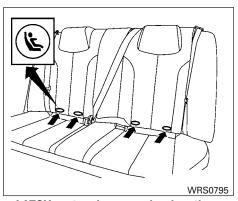
**LATCH** system lower anchor locations LATCH (Lower Anchors and Tethers for CHildren) SYSTEM
