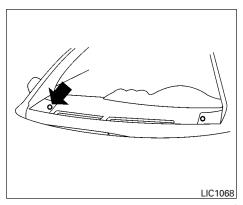
Be sure you do not put anything on top of the autolight sensor located on the top side of the instrument panel. The autolight sensor controls the autolight; if it is covered, the autolight sensor reacts as if it is dark out and the headlights will illuminate. If this occurs while parked with the engine off and the ignition switch placed in the ON position, your vehicle's battery could become discharged.
