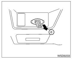
To remove the Intelligent Key from the port, push the ignition switch to the LOCK position and pull the Intelligent Key out of the port (C).
