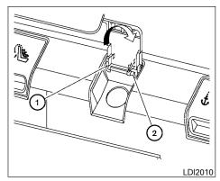
2. Rotate the cover in the direction shown. disengaging the hinge at (1) and slide the second pin from the hinge 2 and remove the cover.
