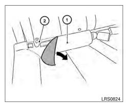
(if so equipped) REAR-FACING CHILD RESTRAINT INSTALLATION USING LATCH
