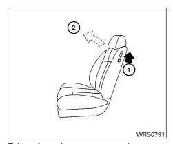
Exiting from the rear seat on the passenger's side, using the upper seatback release lever (if so equipped for Coupe models)
