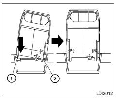
2. With the first pin in position (2), align the second pin with its hinge slot (1) and push down on the cover to completely engage it. A snap sound will be heard.
