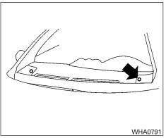
The sunload sensor, located on the top of the instrument panel on the driver's side, helps the system maintain a constant temperature. Do not put anything on or around this sensor.
