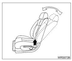
Entry to the rear seat from outside of the vehicle (if so equipped for Coupe models)
