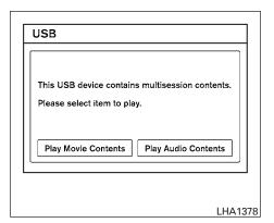
When there are both audio and movie files in the USB memory, the mode select screen is displayed. Use the touchscreen to select the preferred type of file. When there is only type of file in the USB memory, that audio or movie operation screen is displayed and starts to play.
