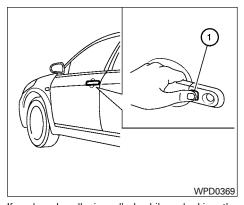
If a door handle is pulled while unlocking the doors, that door may not be unlocked. Returning the door handle to its original position will unlock the door. If the door does not unlock after returning the door handle, push the door handle request switch to unlock the door.
