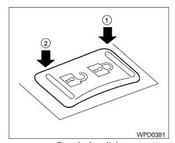
Door lock switch LOCKING WITH POWER DOOR LOCK SWITCH
