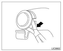
To install the cargo net, attach the net to the retainers.
