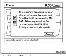
4. When a PIN code appears on the screen, operate the Bluetooth® cellular phone to enter the PIN code.
