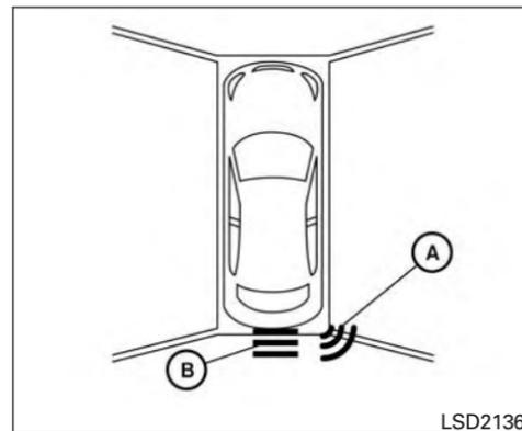
When the corner of the vehicle moves closer to an object, the corner sonar indicators (A) appears. When the center of the vehicle moves close to an object, the center sonar indicator (B) appears.
