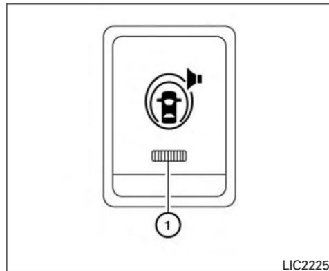
The warning systems switch is used to temporarily turn off the warning systems (Lane Departure Warning (LDW) and Blind Spot Warning (BSW) systems) that are activated using the settings menu in the vehicle information display.
