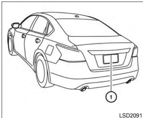
The BSW/LDW systems use the rear view monitor camera unit ① with automatic washer and blower.
