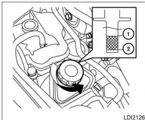
Check the fluid level in the reservoir.
