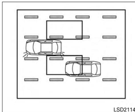
If the driver activates the turn signal, then the Blind Spot indicator light flashes and a chime will sound twice.
