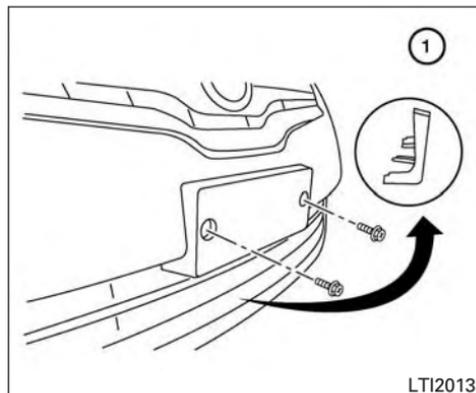
To mount the front license plate, attach the license plate bracket ① to the plastic finisher at the location marks (small dimples) using the two 6 mm screws provided.
