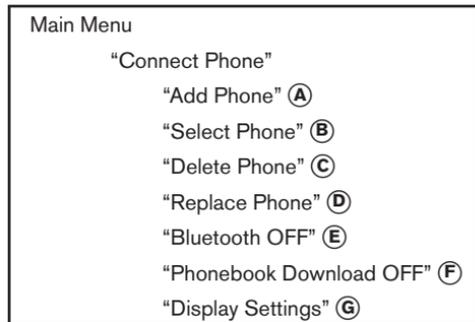
Use the Connect Phone commands to manage the phones connecting to the vehicle or to enable the Bluetooth® function on the vehicle.
