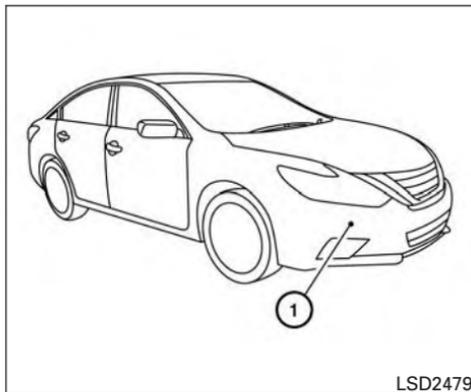
The PFCW system uses a radar sensor **①** located on the front of the vehicle to measure the distance to the vehicle ahead in the same lane.
