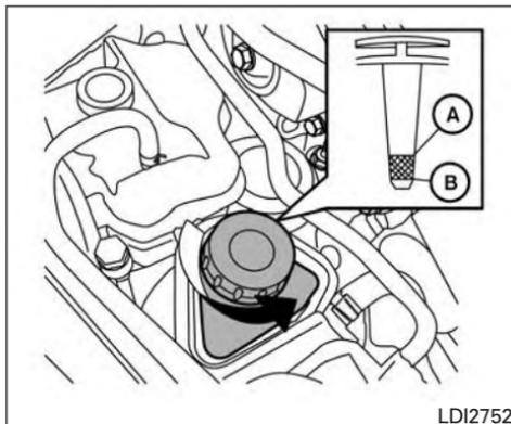
Check the fluid level in the reservoir.
