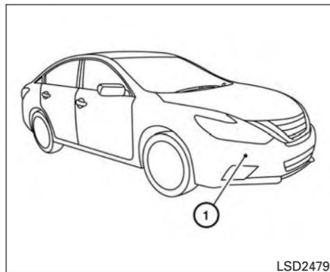
The FEB system uses a radar sensor
