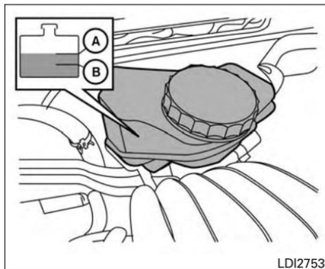
For additional information on brake fluid specification, refer to "Recommended fluids/lubricants and capacities" in the "Technical and consumer information" section of this manual.
