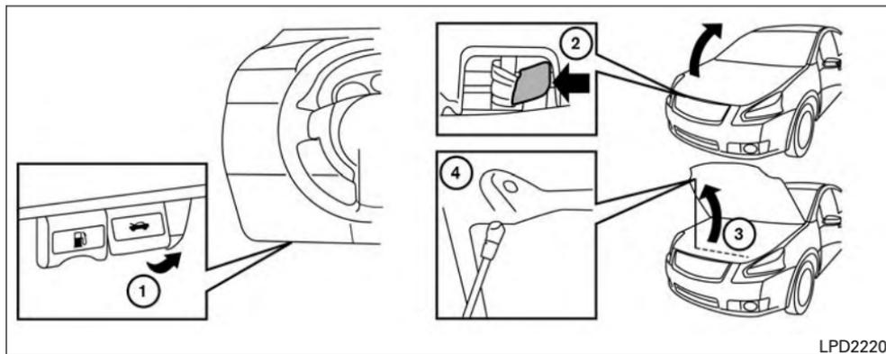
1. Pull the hood lock release handle (1) located below the driver's side instrument panel; the hood springs up slightly.
