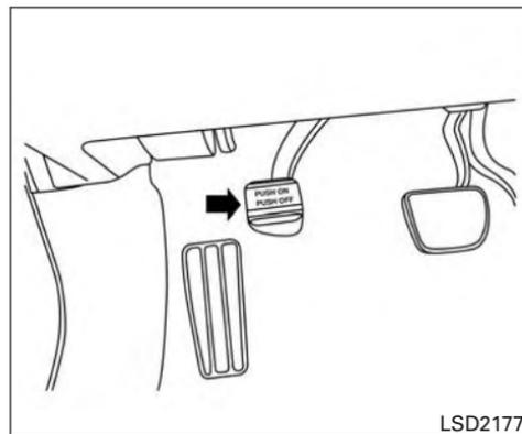
1. To engage, firmly depress the foot brake.
