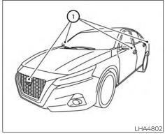
If dirt, rain or snow accumulates on any of the cameras (1), the MOD system may not operate properly. Clean the camera by wiping with a cloth dampened with a diluted mild cleaning agent and then wiping with a drv cloth.
