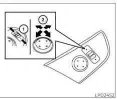
The outside mirror remote control only operates when the ignition switch is placed in the ACC or ON position.
