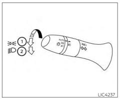
Type C (if so equipped) **HEADLIGHT CONTROL SWITCH**
