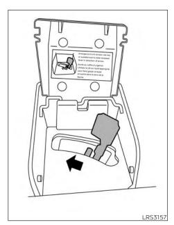
The trunk can be accessed from the driver side and passenger side of the rear seat for loading and unloading, as shown.
