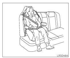
Make sure the child's head will be properly supported by the booster seat or vehicle seat. The seatback must be at or above the center of the child's ears. For example, if a low back booster seat is chosen, the vehicle seatback must be at or above the center of the child's ears If the seatback is lower than the center of the child's ears, a high back booster seat should be used
