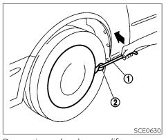
Removing wheel cover (if so equipped)
