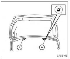
To fold down either side of the rear seat. open the trunk and pull on the knob on that side (A).
