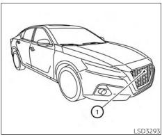
The I-FCW system uses a radar sensor ① located on the front of the vehicle to measure the distance to the vehicle ahead in the same lane.
