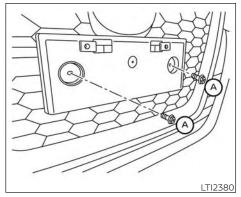
To mount the front license plate, attach the license plate bracket to the bumper fascia at the location marks (small dimples) using the two provided screws (A).
