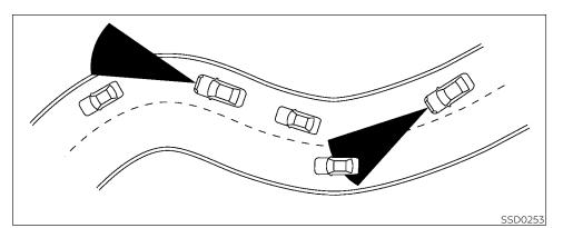
When driving on some roads, such as winding, hilly, curved, narrow roads, or roads which are under construction, the radar sensor may detect vehicles in a different lane, or may temporarily not detect a vehicle traveling ahead. This may cause the radar system to decelerate or accelerate the vehicle.
