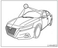
To display the multiple views, the Intelligent Around View Monitor system uses cameras located in the front grille, on the vehicle's outside mirrors and one just above the vehicle's license plate (1).
