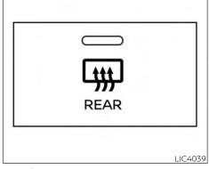
To defrost the rear window glass and outside mirrors (if so equipped), place the ignition switch in the ON position and push the rear window defroster switch on. The rear window defroster indicator light on the switch comes on. Push the switch again to turn the defroster off
