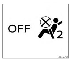
7. If the booster seat is installed in the front passenger seat, place the ignition switch in the ON position. The front passenger air bag status light \*\* \* may or may not illuminate, depending on the size of the child and the type of booster seat being used. For additional information, refer to "Front passenger air bag and status light" in this section.
