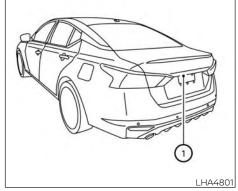
camera (1), the RearView Monitor may not display objects clearly. Clean the camera by wiping it with a cloth dampened with a diluted mild cleaning agent and then wiping it with a dry cloth.
