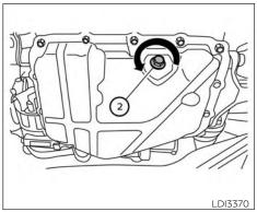
② Oil drain plug (PR25DD)
