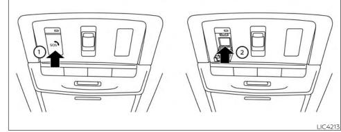
The E-call (SOS) button is used in combination with a NissanConnect® Services subscription to call for assistance in case of an emergency.
