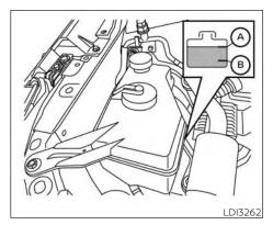
CHECKING ENGINE COOLANT I FV/FI
