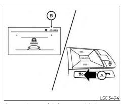
Operating vehicle-to-vehicle distance control mode
