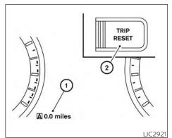
Odometer/Twin trip odometer
