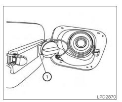
To remove the fuel-filler cap:
