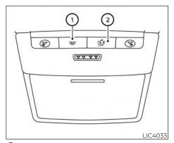
The interior light can be turned ON regardless of door position. The light will go off after a period of time unless the ignition switch is placed in the ON position when any door is opened.
