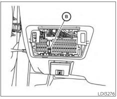
3. Remove the fuse with the fuse puller **B**.
