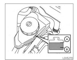
For additional information on brake fluid specification, refer to "Recommended fluids/lubricants and capacities" in the "Technical and consumer information" section of this manual.
