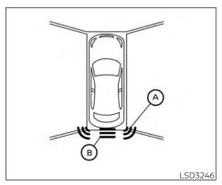
When the corner of the vehicle moves closer to an object, the corner sonar indicator  $\widehat{\mathbf{A}}$  appears. When the center of the vehicle moves close to an object, the center sonar indicator (B) appears.
