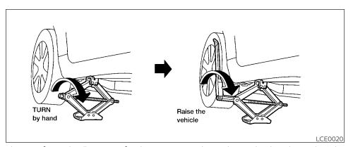
Always refer to the illustration for the correct placement and jack-up points for your specific vehicle model and jack type.
