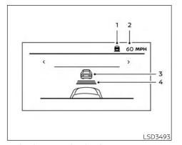
Vehicle-to-vehicle distance control mode display and indicators
