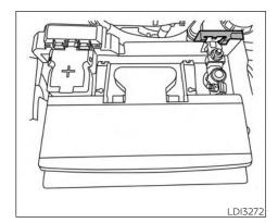
The current sensor is located near the battery along the negative battery cable. If you add electrical accessories to your vehicle, be sure to ground them to a suitable body ground such as the frame or engine block area.
