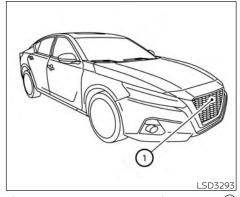
The AEB system uses a radar sensor (1) located on the front of the vehicle to measure the distance to the vehicle ahead in the same lane.
