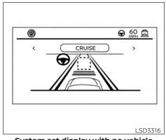
System set display with no vehicle detected ahead No vehicle detected ahead
