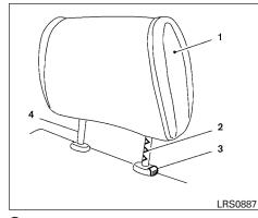
The illustration shows the seating positions equipped with head restraints. The first row head restraints are adjustable.
