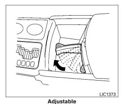
Position the arm on the adjustable cup holder so that the cup is held securely.
