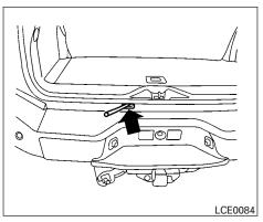
4. Assemble the two straight pieces of the jack rod. Find the oval-shaped opening above the middle of the license plate. Pass the T-shaped end of the jack rod through the opening and direct it toward the spare tire winch, located directly above the spare tire.
