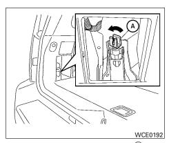
3. Unscrew the rotating mechanism (A) counterclockwise until loosened on cradle. Remove the jack.
