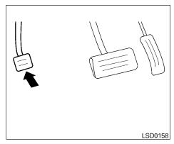
**To engage:** Firmly depress the parking brake.
