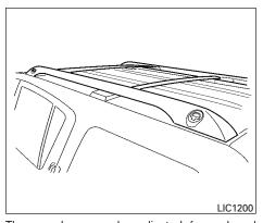
The crossbars can be adjusted forward and backward. Loosen the thumbwheel ① and adjust the crossbar to the desired position. Tighten the thumbwheel. Place your luggage on the bars and secure the luggage with rope to the utility loops ②. Do not place luggage on the side rails or tie rope directly to the side rails. Always be sure the thumbwheels are fully tightened to keep the crossbar in place. Do not use utility loops for any purpose other than securing luggage.
