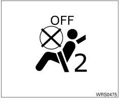
7. If the booster seat is installed in the front passenger seat, place the ignition switch in the ON position. The front passenger air bag status light R may or may not illuminate, depending on the size of the child and the type of booster seat being used. See "Front passenger air bag and status light" later in this section.
