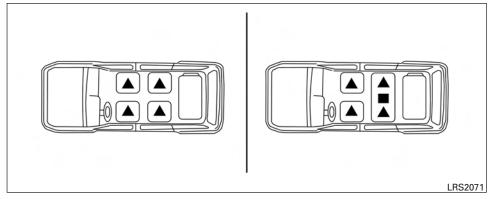
The illustration shows the seating positions equipped with head restraints. The second row head restraints are removable but not adjustable.
