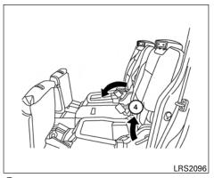
Then lift up on the recline lever to fold the seatback flat forward.
