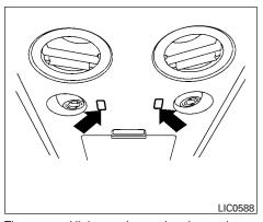
The personal lights on the overhead console can be swiveled 360 degrees. To turn on the light, press the button. Press the button again to turn off the light.
