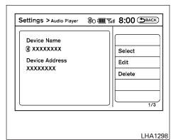
6. The Device Name and Device Address are displayed on the screen. Select the "Select" key to make this device the active Bluetooth® audio player. Select the "Edit" key to edit the details of the player, such as Device Name. Select the "Delete" key to delete the device.
