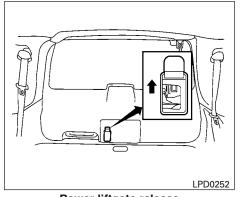
Power liftgate release Power liftgate (if so equipped)
