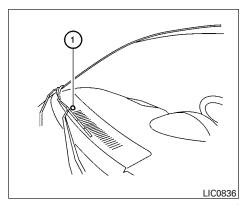
Be sure you do not put anything on top of the autolight sensor ① located in the top side of the instrument panel. The autolight sensor controls the autolight; if it is covered, the autolight sensor reacts as if it is dark out and the headlights will illuminate. If this occurs while parked with the engine off and the ignition switch placed in the ON position, your vehicle's battery could become discharged.
