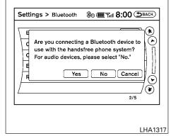
A screen will appear asking if you are connecting the device to use with the handsfree phone system. Select the "No" key.
