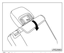
③ Pull the strap to release the head restraint rearward.
