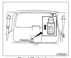
Manual liftgate release Manual liftgate (if so equipped)
