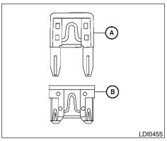
Two types of fuses are used. Type (A) is used in the fuse boxes in the engine compartment. Type (B) is used in the passenger compartment fuse hox.
