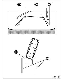
3. Slowly back up the vehicle adjusting the steering wheel so that the predicted course lines (B) enter the parking space (C).
