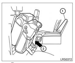
Then (2) lift up on the lower corner of the seat base and tip the 2nd row captain's chair forward. To exit the 3rd row bench seat, lift up on the same seatback latch and fold the seatback forward onto the seat base. Then lift up on the seat base and tip it forward.
