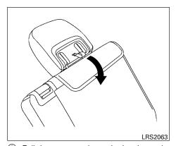
② Pull the strap to release the head restraint rearward.
