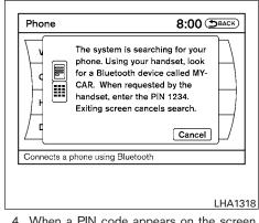
When a PIN code appears on the screen, operate the Bluetooth® cellular phone to enter the PIN code.
