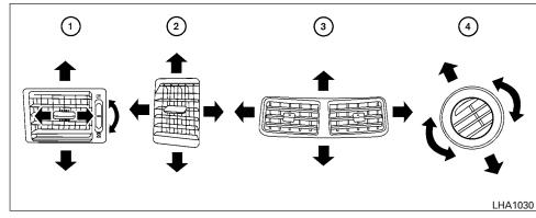
Adjust air flow direction for the driver's and passenger's side vents ①, center vents ②, and rear passengers' vents (3) and (4) by moving the vent slide and/or vent assemblies.
