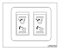
To fold down the 3rd row seats, push and hold the bottom portion of the switch.
