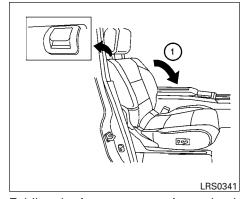
Folding the front passenger's seatback (if so equipped)
