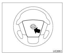
To sound the horn, push near the horn icon of the steering wheel.
