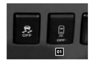
■ Turn the system off by pushing the Rear Sonar System off switch of . Push the switch again to activate the system.
