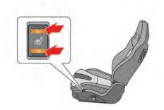
The seat heaters can be used when the ignition switch is in the ON position. The front seats are warmed by the built-in heaters.
