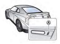
When you carry the Intelligent Key with you, you can lock or unlock all doors by pushing the door handle request switch (A) within the range of operation.
