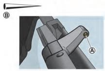
Be careful not to clog the washer nozzle (A). This may cause improper windshield washer operation. If the nozzle is clogged, remove any objects with a needle or small pin (B). Be careful not to damage the nozzle.
