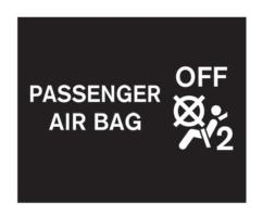
7. If the booster seat is installed in the front passenger seat, push the ignition switch to the ON position. The front passenger air bag status light "" may or may not illuminate depending on the size of the child and the type of booster seat used. ( "Front passenger air bag and status light" page 1-41)
