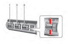
The control of the dual clutch transmission. Bilstein DampTronic® electronically controlled shock absorbers and Vehicle Dynamic Control (VDC) can be changed to the desired modes by operating the setup switches. Select the desired mode best suited to the driving conditions.
