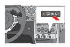
To defog/defrost the rear window, start the engine and push the switch on. The indicator light on the switch will come on. Push the switch again to turn the defroster off.
