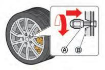
5. Remove the wheel nuts and then remove the wheel.
