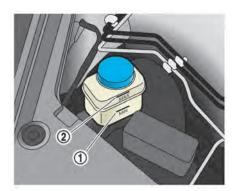
Check the fluid level in the reservoir. If the fluid is below the MIN line ① or the brake warning light comes on, add Genuine NISSAN Brake Fluid R35 Special II fluid up to the MAX line ②. If fluid must be added frequently, the system should be checked by a GT-R certified NISSAN dealer.
