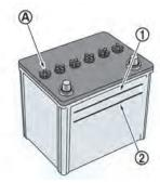
Check the fluid level in each cell (Remove the battery cover if it is necessary). It should be between the UPPER LEVEL ① and LOWER LEVEL ② lines.
