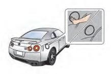
2. Press the rear side of the fuel-filler door to release the door lock, and open the door.
