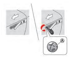
With the outside door handle lifted up, use the mechanical key and turn the key cylinder cap (A) counterclockwise to remove.
