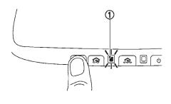
2. Using both hands, simultaneously press and hold the desired HomeLink® button and handheld transmitter button. DO NOT release until the HomeLink® indicator light (1) flashes slowly and then rapidly. When the indicator light flashes rapidly, both buttons may be released. (The rapid flashing indicates successful programming.)
