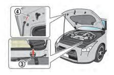
3. Grasp the insulated part of the stay ③ and release it from the hook, then securely insert it into the hood hole ④.
