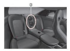
This system uses the front and rear microphones (1) to detect engine booming noise. The system then automatically generates a noise cancelling sound through the speakers (2) and woofer (3) to reduce engine booming noise.
