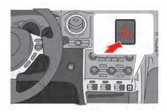
Push the switch on to warn other drivers when you must stop or park under emergency conditions. All turn signal lights will flash.
