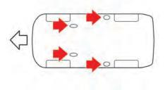
Do not use the tie down hooks for towing or vehicle recovery.
