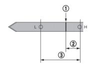
NISSAN recommends to adjust the engine oil level ① to be 0.39 in (10 mm) (1/8 gal (0.5 liters)) ② below the H mark on the engine oil dipstick. (③ range is 1.18 in (30 mm).) Before checking the oil level, run the engine until it reaches operating temperature and wait at least 5 minutes after turning off the engine. Make sure the oil level always remains above the L mark.
