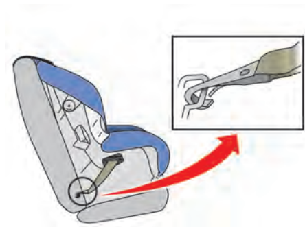
LATCH webbing-mounted attachment
