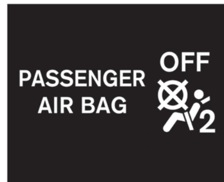
Front passenger air bag status light
