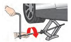
4. Carefully raise the vehicle until the tire clears the ground. To lift the vehicle, securely hold the jack lever and rod with both hands as shown above.
