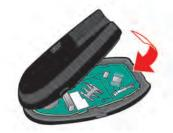
Reconnect the upper and lower parts of the Intelligent Key.
