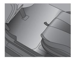
3. Make sure the floor mat does not interfere with pedal operation. With the ignition in the OFF position and the shift lever in the P (Park) position, fully apply and release all pedals. The floor mat must not interfere with pedal operation or prevent the pedal from returning to its normal position. It is recommended you see a GT-R certified NISSAN dealer for details about installing the floor mats in your vehicle.
