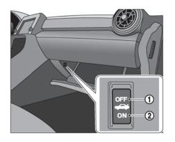
valet and keep the mechanical key with you. ( \*\* "Valet hand-off" page 3-3) To connect the power to the trunk lid, push the switch to the ON position 2.
