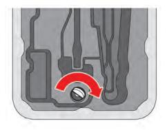
2. Insert the mechanical key into the emergency trunk lid opener and turn it clockwise until it stops.
