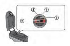
Start the engine and check that the indicator ① (green) is illuminating. The indicator ① (green) illuminates when GPS information is received.
