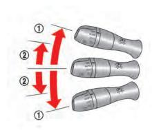
turn signal begins to flash, but the lever does not latch, and release the lever. The turn signal will automatically flash three times.
