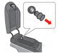
Inside the console box (except for NISMO models) Open the cap to use the outlet. Close the cap after use.
