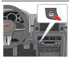
To defog/defrost the rear window, start the engine and push the switch on. The indicator light on the switch will come on. Push the switch again to turn the defroster off.
