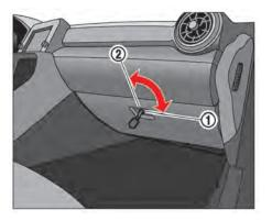
Use the mechanical key to lock ① and unlock ② the glove box. ( The "Mechanical" key" page 3-3)
