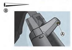
Be careful not to clog the washer nozzle (A). This may cause improper windshield washer operation. If the nozzle is cloqged, remove any objects with a needle or small pin (B). Be careful not to damage the nozzle.
