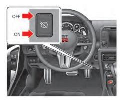
To close the electronic control valve, push the exhaust sound control switch to the ON side.
