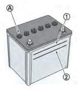
Check the fluid level in each cell (Remove the battery cover if it is necessary). It should be between the UPPER LEVEL (1) and LOWER LEVEL @ lines.
