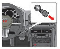
Next to the steering wheel Pull out the cap to use the outlet. Replace the cap after use.
