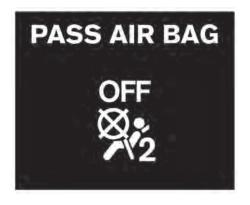
7. If the booster seat is installed in the front passenger seat, push the ignition switch to the ON position. The front passenger air bag status light may or may not illuminate depending on the size of the child and the type of booster seat used. ( Front passenger air bag and status light" page 1-42)
