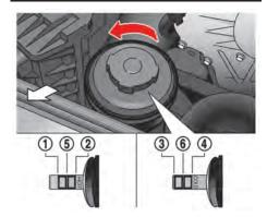
Check the fluid level in the reservoir Remove the cap that is attached with a gauge inside.
