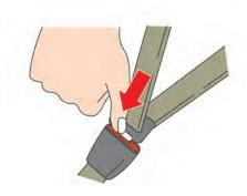
Grasp the shoulder belt and pull forward quickly. The retractor should lock and restrict further belt movement.
