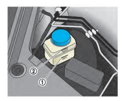
Check the fluid level in the reservoir. If the fluid is below the MIN line ① or the brake warning light comes on, add Genuine NISSAN Brake Fluid R35 Special II fluid (or equivalent) up to the MAX line 2. If fluid must be added frequently, the system should be checked by a GT-R certified NISSAN dealer.
