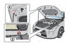
3. Grasp the insulated part of the stay ③ and release it from the hook, then securely insert it into the hood hole 4.
