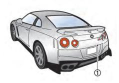
To display the rear view, the RearView Monitor system uses a camera ① located just above the vehicle's license plate.
