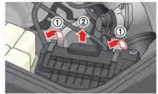
Remove the retainers (1) as illustrated and pull out the filter element 2.
