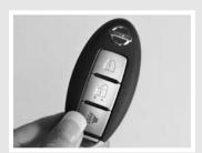
■ To open the liftgate, push the liftgate opener switch and pull up.
