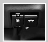
The fuel-filler door is located on the right, rear side of the vehicle.
