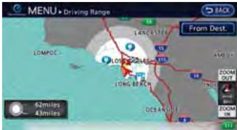
By pressing the
