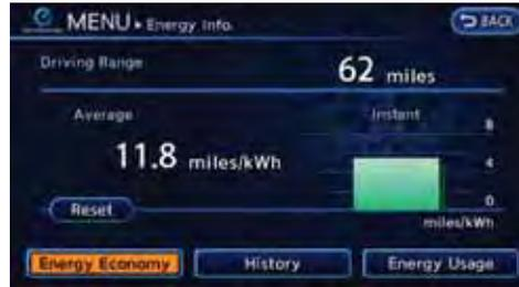
Estimated driving range and energy usage of various systems are displayed. Also, variation of the estimated driving distances between the climate control ON and OFF is displayed.
