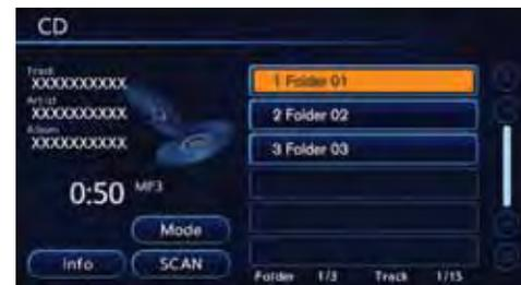
Push the **CD-AUX** button to turn on the audio system and display the audio screen. Push the **CD-AUX** button to toggle the mode: iPod player/USB memory→CD→Bluetooth® streaming audio\*1→AUX.
