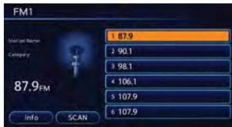
Push the **FM-AM** button to turn on the radio and display the radio screen. Push the switch to toggle the radio mode: AM→FM1→FM2.
