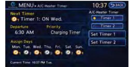
The air conditioner starts to operate at the time of day and day of the week specified in the settings. This pre cools or heats the passenger compartment before starting to drive. Electric power consumption from the Li-ion battery resulting from heater and air conditioner operation can be reduced because the temperature in the passenger room is adjusted before starting to drive.
