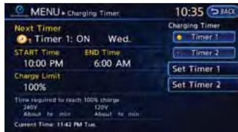
Charging of the Li-ion battery will automatically start at a scheduled time according to the start time, end time and day of the week set. The timer charge function allows two different timer settings. Each timer charge can be set to activate on a different day of the week. If no timer is set, the charge will start immediately after connecting the charge connector.
