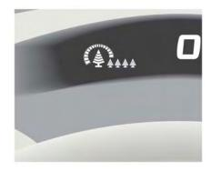
While the vehicle is being driven you can check your own ECO drive level on the ECO indicator. See "ECO indicator" in the "2. Instruments and controls" section.
