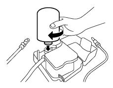
4. Remove the cap from the tire valve on the flat tire.
