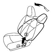
The reclining feature allows adjustment of the seatback for occupants of different sizes for added comfort and to help obtain proper seat belt fit. See "Precautions on seat belt usage" later in this section. Also, the seatback can be reclined to allow occupants to rest when the vehicle is stopped and the vehicle is in the P (Park) position or N (Neutral) position with the parking brake applied.
