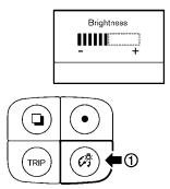
The instrument brightness control switch can be operated when the power switch is in the ON position. When the switch is operated, the dot matrix liquid crystal display switches to the brightness adjustment mode.
