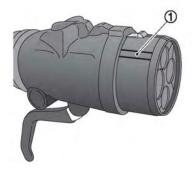
4. Align ① with the groove of the charge port and insert the charge connector.
