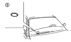
Be sure not to put anything on top of the photo sensor (1) located on the top of the instrument panel. The photo sensor controls the autolight; if it is covered, the photo sensor reacts as if it is dark and the headlights will illuminate.
