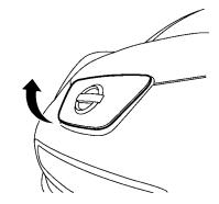
2. Put your hand into the under side of the lid and open until it is in the fully open position.
