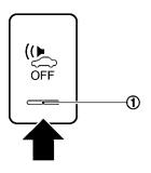
The Approaching Vehicle Sound for Pedestrians (VSP) system is a function that uses sound to help alert pedestrians of the presence of the vehicle when it is being driven at a low speed.
