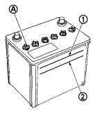
Check the fluid level in each cell. It should be between the UPPER LEVEL (1) and LOWER LEVEL (2) lines.
