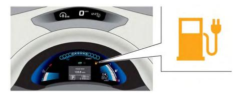
If the low battery charge warning light illuminates, the Li-ion battery charge is too low for travel. See "Low battery charge warning light" in the "2. Instruments and controls" section. Charge the Li-ion battery as soon as possible.
