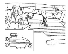
Check the fluid level in the reservoir. If the fluid is below the MIN line (1) or the brake warning light illuminates, add Genuine NISSAN Super Heavy Duty Brake Fluid or equivalent DOT 3 fluid up to the MAX line (2). If fluid must be added frequently, the system should be checked by a NISSAN certified LEAF dealer.
