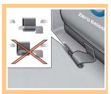
Pass the lower side belt of the EVSE (Electric Vehicle Supply Equipment) case securely through the fastener on the bottom of the luggage board. If the case suddenly becomes loose, it may cause serious injury or death.
