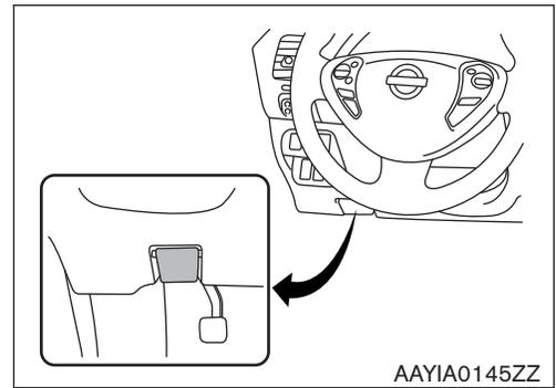
2. Press and expand the pawls (A) on the sides of the fuse box and remove the fuse box (1) from its housing.
