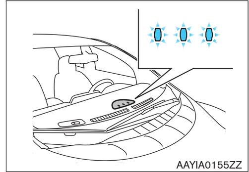
Before disconnecting the 12-volt battery terminal, if necessary, lower the windows, unlock the doors, and open the rear hatch as required. Once 12-volt battery is disconnected, power controls will not operate.
