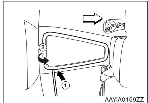
2. Remove the 10 mm access cover bolts (1) and remove the cover (2).
