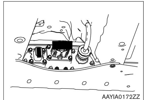
5. Disconnect the high-voltage battery vehicle communications connector (A) while turning it counterclockwise.
