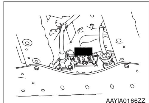
4. Disconnect the cabin heater harness connector (A) from the high-voltage battery.
