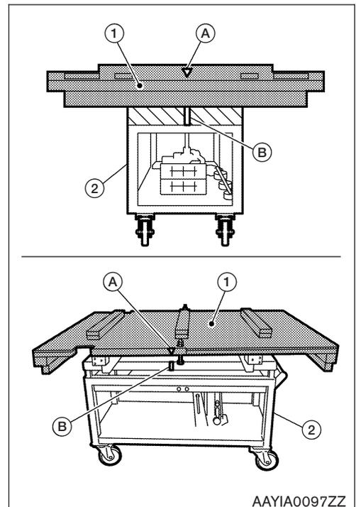
9. Set the pallet (1) under the high-voltage battery.
