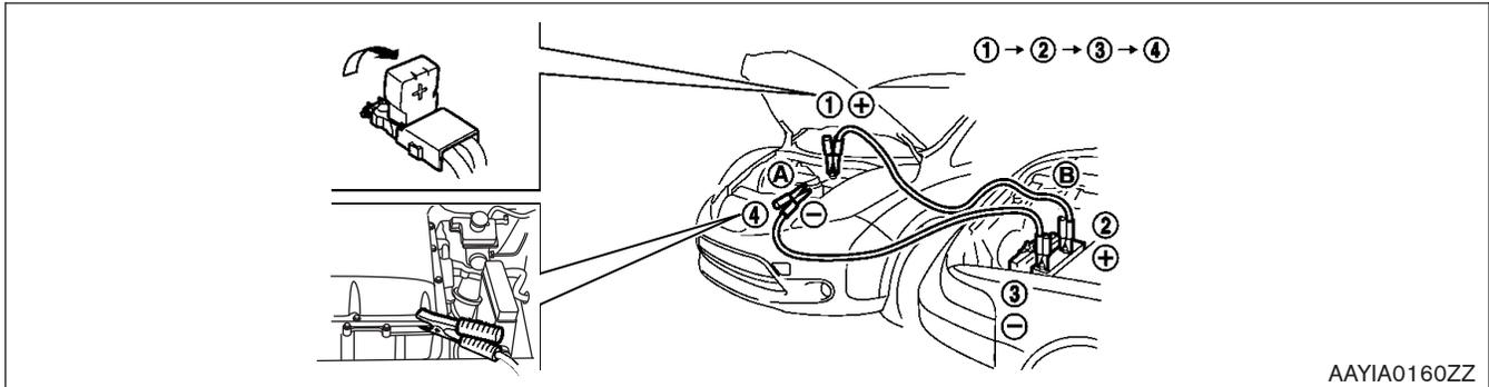
1. If the booster battery is in another vehicle (B), position the two vehicles (A and B) to bring their 12-volt batteries into close proximity to each other.
