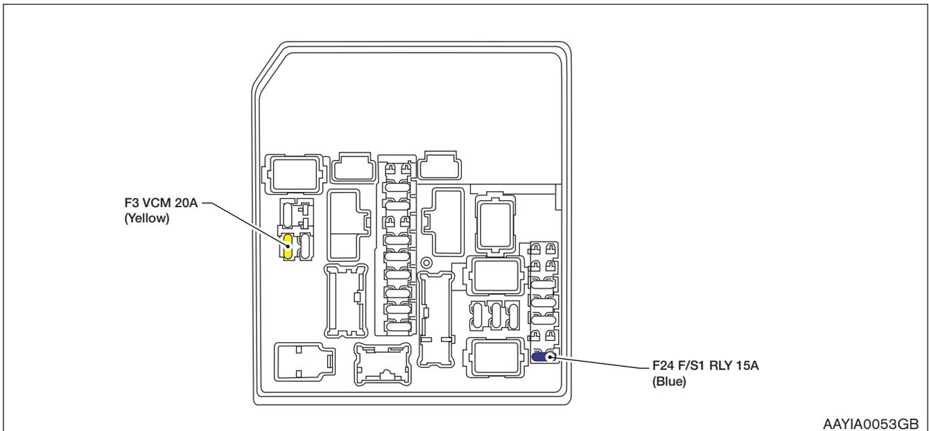
4. Remove the fuse box cover and remove the 20A VCM fuse.
