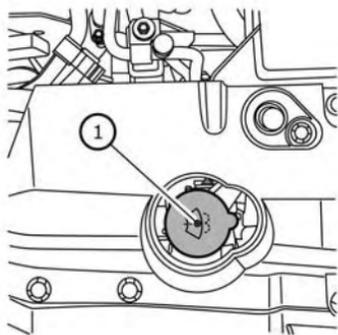
To check the fluid level, use your finger to plug the center hole ① of the cap/tube assembly, then remove it from the reservoir. If there is no fluid in the tube, add fluid.
