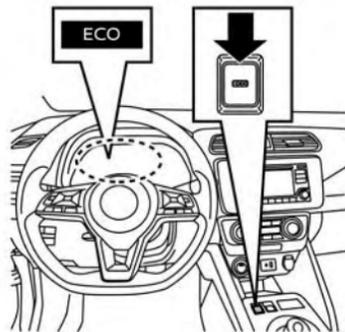
The ECO mode helps reduce power consumption by reducing acceleration when compared to the same accelerator pedal position in the D (Drive) position. Use the ECO mode for maximum driving range and for city driving.
