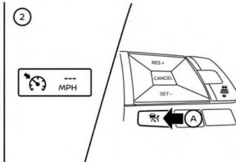
**Selecting the conventional (fixed speed) cruise control mode:** To choose the conventional (fixed speed) cruise control mode ②, push and hold the ICC switch (A) for longer than approximately 1.5 seconds. For additional information, refer to “Conventional (fixed speed) cruise control mode” in this section.
