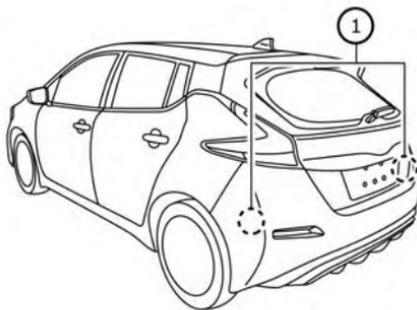
The BSW system uses radar sensors ① installed near the rear bumper to detect other vehicles in an adjacent lane.
