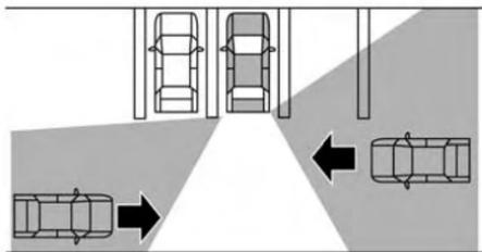
The RCTA system uses radar sensors ① installed on both sides near the rear bumper to detect an approaching vehicle.
