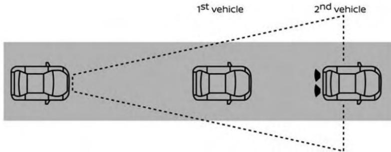
The I-FCW system operates at speeds above approximately 3 mph (5 km/h).
