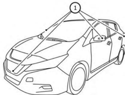
To display the multiple views, the Intelligent Around View Monitor system uses cameras located in the front grille, on the vehicle's outside mirrors and one just above the vehicle's license plate ①.
