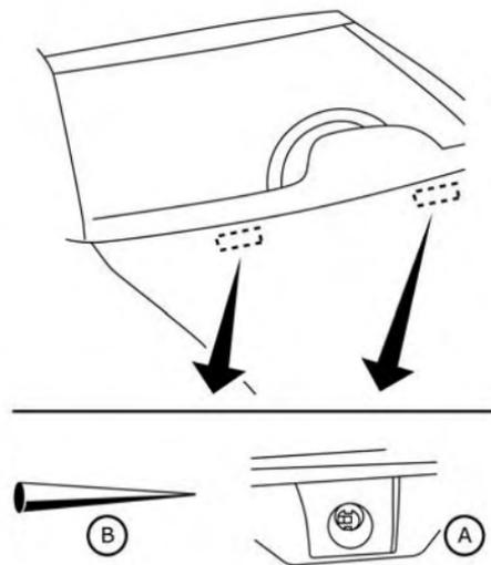
Be careful not to clog the washer nozzle (A). This may cause improper windshield washer operation. If the nozzle is clogged, remove any objects with a needle or small pin (B). Be careful not to damage the nozzle.
