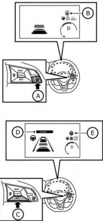
1. Push the ProPILOT Assist switch (A). This turns on the ProPILOT Assist system and displays the status of the ProPILOT Assist system on the vehicle information display (B).
