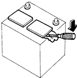
1. Remove the vent caps with a screwdriver as shown. Use a cloth to protect the battery case.
