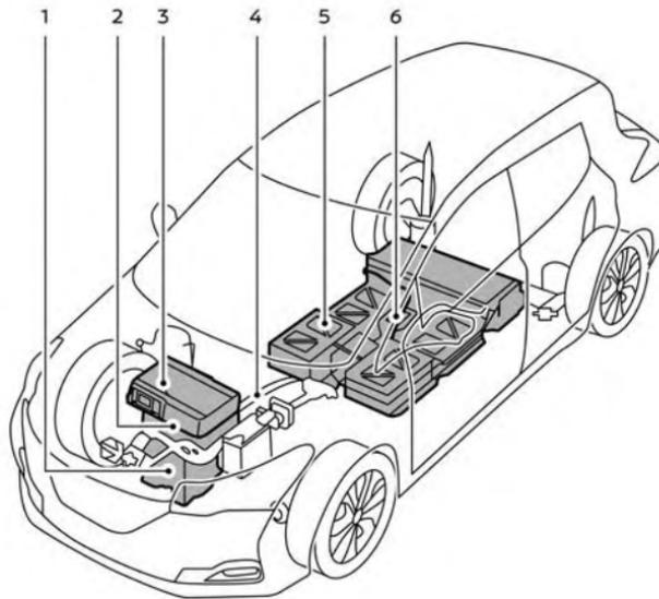
1. Traction motor and reduction gear
