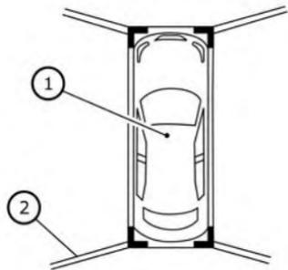
After the EV system is placed in the ON position, the non-viewable areas ② are highlighted in yellow for several seconds after the bird's-eye view is displayed. It will be shown only the first time after the power switch is placed in the ON position.
