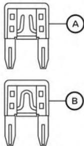
6. If the fuse is open (A), replace it with a new fuse (B).
