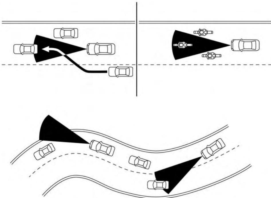
When driving on some roads, such as winding, hilly, curved, narrow roads, or roads which are under construction, the radar sensor may detect vehicles in a different lane, or may temporarily not detect a vehicle traveling ahead. This may cause the radar system to decelerate or accelerate the vehicle.
