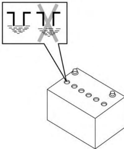
2. Check the fluid level in each cell. If it is necessary to add fluid, add only distilled water to bring the level up to the bottom of the filler opening. **Do not overfill.** Reinstall the vent caps.
