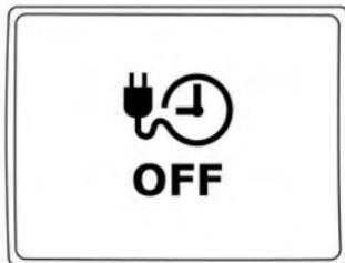
To turn off the charge timer, push the immediate charge switch. For additional information, refer to "Charging timer" in the "Charging" section of this manual.
