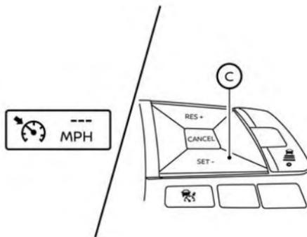
To set cruising speed, accelerate your vehicle to the desired speed, push the SET- (C) switch and release it. (The color of the cruise indicator changes to green and set vehicle speed indicator comes on.) Take your foot off the accelerator pedal. Your vehicle will maintain the set speed.
