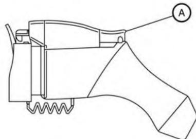
6. Open the charge port cap. For additional information, refer to "Charge port cap" in the "Pre-driving checks and adjustments" section of this manual.
