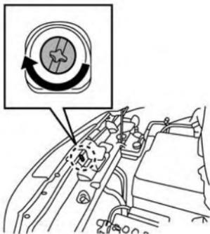
If the charge connector cannot be unlocked
