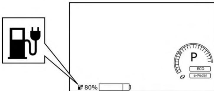
If the low battery charge indicator
