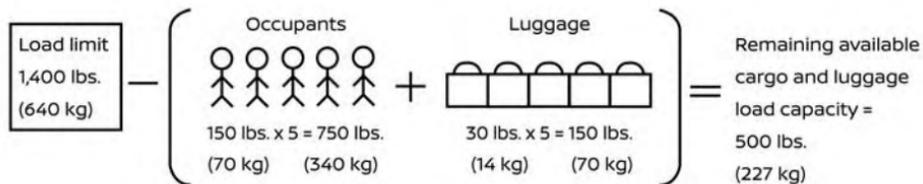
Steps for determining correct load limit
