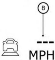
When passing another vehicle, the set speed indicator **B** flashes when the vehicle speed exceeds the set speed. The vehicle ahead detection indicator turns off when the area ahead of the vehicle is open. When the pedal is released, the vehicle returns to the previously set speed. Even though your vehicle speed is set in the ICC system, you can depress the accelerator pedal when it is necessary to accelerate your vehicle rapidly.
