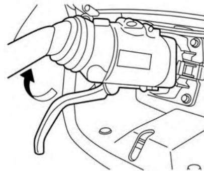
5. Grasp the lock lever and lock the charge connector.
