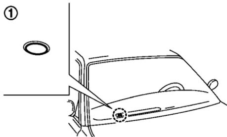
Be sure not to put anything on top of the photo sensor ① located on the top of the instrument panel. The photo sensor controls the autolight; if it is covered, the photo sensor reacts as if it is dark and the headlights will illuminate.
