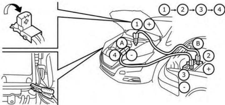
1. If the booster battery is in another vehicle (B), position the two vehicles (A) and (B) to bring their 12-volt batteries into close proximity to each other.
