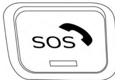
The E-call (SOS) system button is used in combination with a NissanConnect® (for Leaf) Services subscription to call for assistance in case of an emergency.
