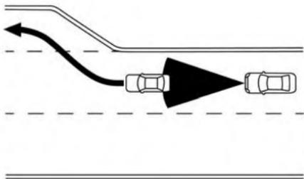
The vehicle may not maintain the set speed on winding or hilly roads. If this occurs, you will have to manually control the vehicle speed.
