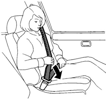
3. Position the lap belt portion **low and snug on the hips** as shown.
