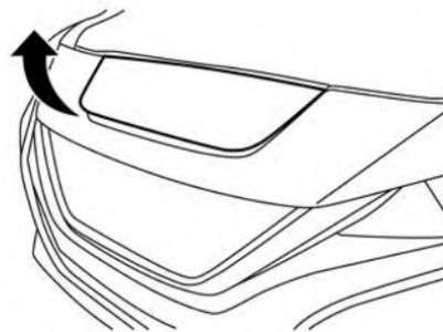
2. Put your hand into the underside of the lid and open until it is in the fully open position.
