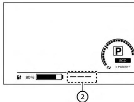
2. If the vehicle is driven and the Li-ion battery continues to discharge, the driving range on the instrument panel changes to “---” ②.
