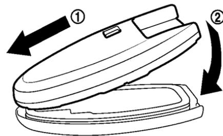
4. Align the tips of the upper and lower parts ①, and then push them together ② until it is securely closed.
