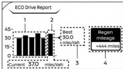
If the vehicle has been driven mostly on downhill roads, more energy is regenerated. This may cause the regenerated energy (mileage) (4) to show a longer distance than the vehicle was driven or the current energy economy (2) to show "99.9 miles/kWh."
