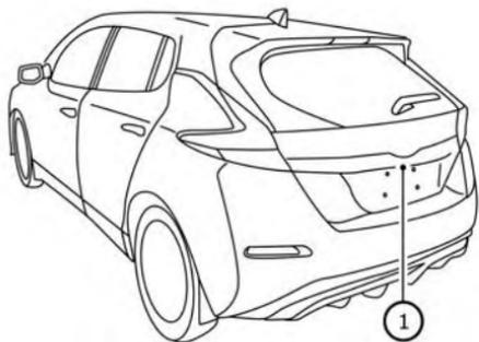
If dirt, rain or snow accumulates on the camera ①, the RearView Monitor may not display objects clearly. Clean the camera by wiping it with a cloth dampened with a diluted mild cleaning agent and then wiping it with a dry cloth.
