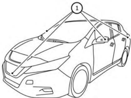
If dirt, rain or snow accumulates on any of the cameras ①, the Intelligent Around View Monitor may not display objects clearly. Clean the camera by wiping with a cloth dampened with a diluted mild cleaning agent and then wiping with a dry cloth.
