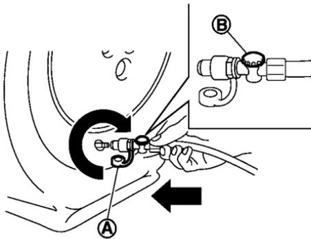
6. Push the power switch to the ACC position. Then turn the compressor switch to the ON (-) position and inflate the tire up to the pressure that is specified on the Tire and Loading Information label affixed to the driver's side center pillar if possible, or to the minimum of 26 psi (180 kPa). Turn the air compressor off briefly in order to check the tire pressure with the pressure gauge.
