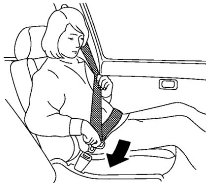
2. Slowly pull the seat belt out of the retractor and insert the tongue into the buckle until you hear and feel the latch engage.
