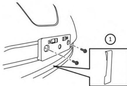
To mount the front license plate, attach the license plate bracket ① to the bumper fascia at the location marks (small dimples) using the two provided screws.
