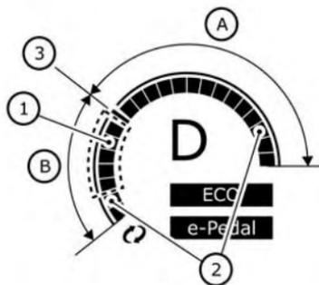
The white illuminated portion (1) moves to the left when power is generated and provided to the Li-ion battery by the regenerative brake system (Li-ion battery charging).
