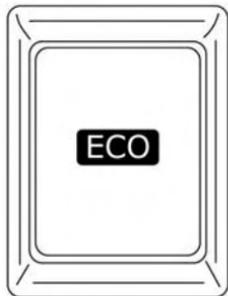
To turn on the ECO mode, push the ECO switch. The ECO mode indicator appears on the meter.
