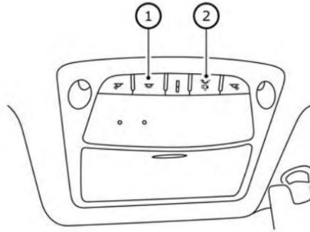
The interior lights can be turned on ① regardless of door position. The lights will go off after a period of time unless the power switch is placed in the ON position when any door is opened.
