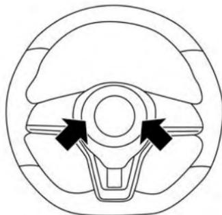
To sound the horn, push the center pad area of the steering wheel.
