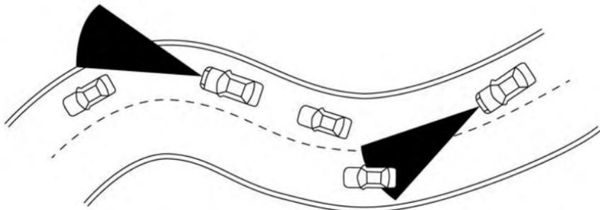
When driving on some roads, such as winding, hilly, curved, narrow roads, or roads which are under construction, the ICC sensor may detect vehicles in a different lane, or may temporarily not detect a vehicle traveling ahead. This may cause the ICC system to decelerate or accelerate the vehicle.
