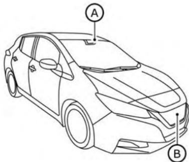
The AEB with Pedestrian Detection system can assist the driver when there is a risk of a forward collision with the vehicle ahead in the traveling lane or with a pedestrian ahead in the traveling lane.
