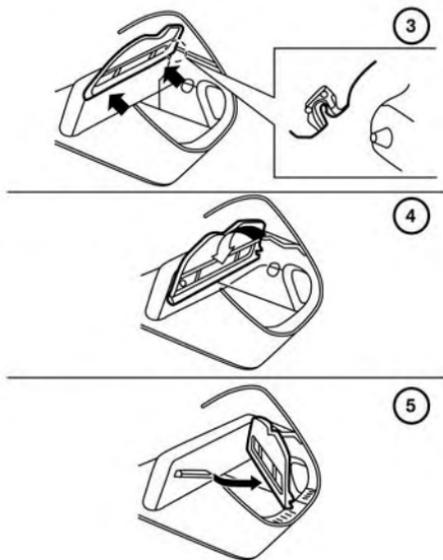
4. Slide down the tonneau cover along the rear seat back.
