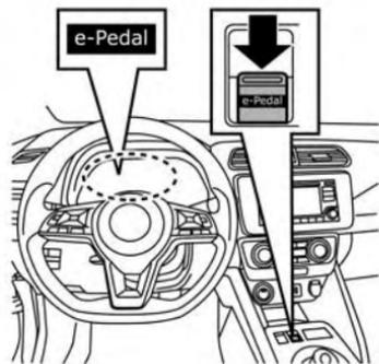
To activate or deactivate the e-Pedal system, place the power switch in the ON position and pull the e-Pedal switch located on the center console. The e-Pedal system turns on or off each time the e-Pedal switch is pulled. (The e-Pedal indicator in the vehicle information display shows the status of the e-Pedal system.)
