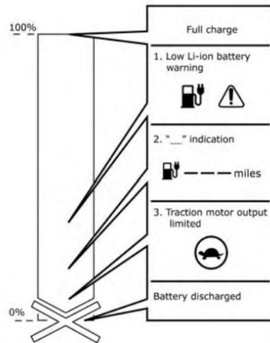
1. The following warning lights illuminate on the instrument panel and messages are displayed on the vehicle information display at the same time to indicate low Li-ion battery charge:
