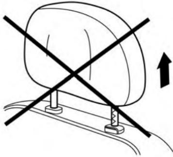
Make sure the head restraint/headrest is positioned so the lock knob is engaged in the notch before riding in that designated seating position.
