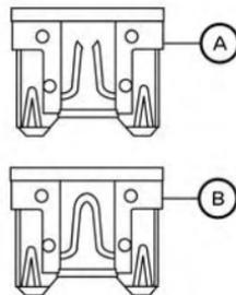
5. If the fuse is open (A), replace it with a new fuse (B).
