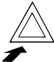
Push the switch on to warn other drivers when you must stop or park under emergency conditions. All turn signal lights will flash.
