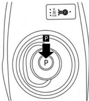
ing the foot brake pedal depressed then push the P (Park) position switch and place the vehicle in the P (Park) position. For additional information, refer to "Parking brake" in this section.
