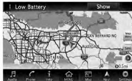
1. The notification is displayed on the upper left side of the STATUS screen. Touch [Show] to display the screen showing detailed information.
