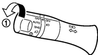
To turn the autolight system off, turn the switch to the OFF,
