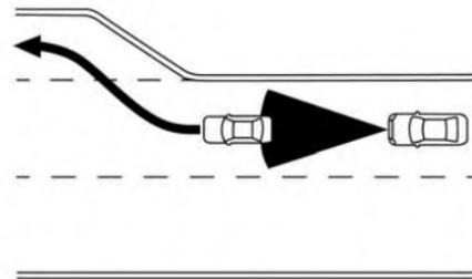
When driving on the freeway at a set speed and approaching a slower traveling vehicle ahead, the ICC system will adjust the speed to maintain the distance, selected by the driver, from the vehicle ahead. If the vehicle ahead changes lanes or exits the freeway, the ICC system will accelerate and maintain the speed up to the set speed. Pay attention to the driving operation to maintain control of the vehicle as it accelerates to the set speed.
