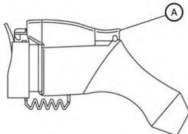
8. Connect the charge connector to the charge port. If it is connected normally, a beep will sound once.
