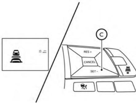
**To set cruising speed,** accelerate your vehicle to the desired speed, push the SET-switch (C) and release it. The ICC system set indicator (green), vehicle ahead detection indicator, set distance indicator and set vehicle speed indicator (B) will come on. Take your foot off the accelerator pedal. Your vehicle will maintain the set speed.
