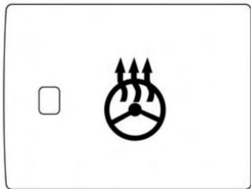
The heated steering wheel system is designed to operate only when the surface temperature of the steering wheel is below approximately 68°F (20°C).
