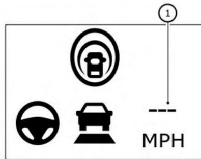
When the SET- switch is pushed under the following conditions, the ProPILOT Assist system cannot be set and the set vehicle speed indicator ① blinks for approximately 2 seconds:
