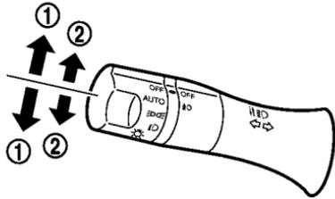
Move the lever up or down until the turn signal begins to flash, but the lever does not latch, and release the lever. The turn signal will automatically flash three times.
