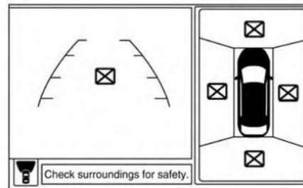
When the "[X]" icon is displayed on the screen, the camera image may be receiving temporary electronic disturbances from surrounding devices. This will not hinder normal driving operation but the system should be inspected if it occurs frequently. It is recommended that you visit a NISSAN certified LEAF dealer for this service.
