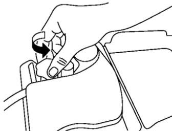
2. Take the hose ① and the power plug ② out of the air compressor. Remove the cap of the bottle holder from the air compressor.
