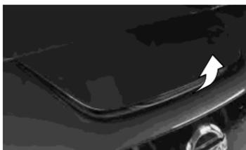
**AUTO** – The charge connector is locked while charging is in progress and unlocked automatically when charging is complete.
