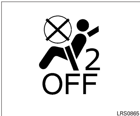
Front passenger air bag and status light
