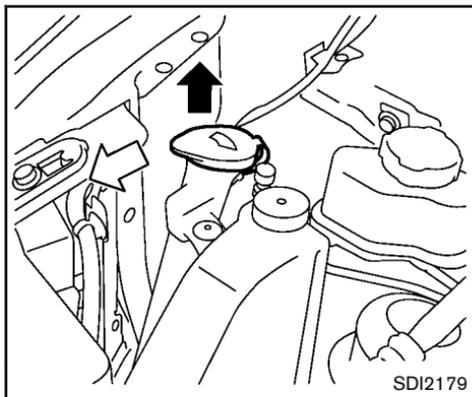
Fill the window washer fluid reservoir periodically. Add window washer fluid when the low window washer fluid warning light illuminates.
