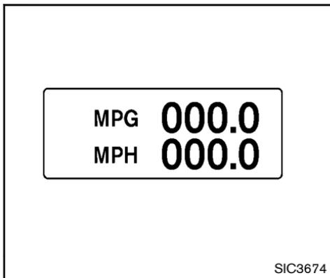
done by pushing the ● switch (B) for longer than 1 second. (The average fuel consumption is also reset at the same time.)
