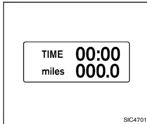
Elapsed time and trip odometer (miles or km)
