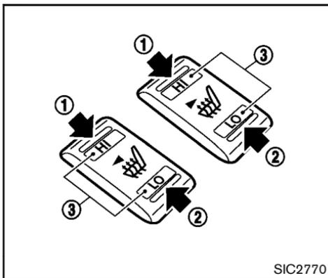
The seats are warmed by built-in heaters. The switches located on the center console and rear doors (if so equipped for rear seats) can be operated independently of each other.
