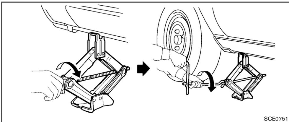
2. Loosen each wheel nut one or two turns by turning counterclockwise with the wheel nut wrench. **Do not remove the wheel nuts until the tire is off the ground.**
