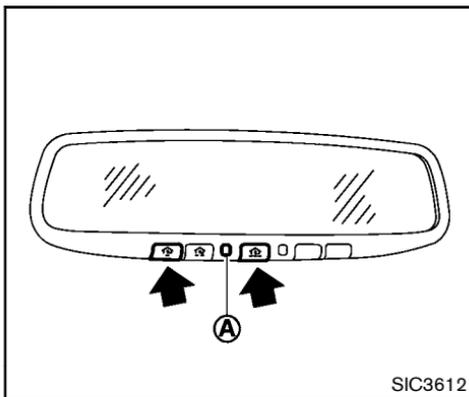
1. To begin, push and hold the 2 outer HomeLink® buttons (to clear the memory) until the indicator light (A) blinks (after 20 seconds). Release both buttons.
