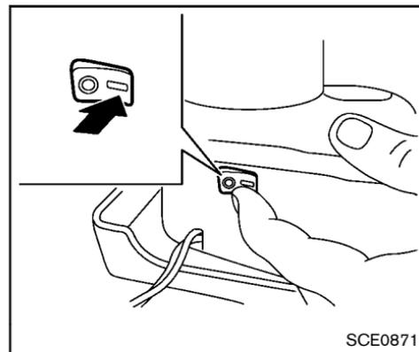
3. Remove the cap from the tire sealant bottle, and screw the bottle clockwise onto the bottle holder. (Leave the bottle seal intact. Screwing the bottle onto the bottle holder will pierce the seal of the bottle.)
