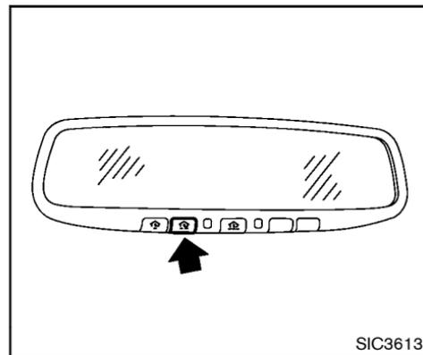
3. Using both hands, simultaneously push and hold both the HomeLink® button you want to program and the hand-held transmitter button.
