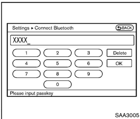
4. Choose a PIN code to use with the compatible Bluetooth audio device using the number input screen. The PIN code will need to be entered into the Bluetooth® audio device after step 5. Select the "OK" key.
