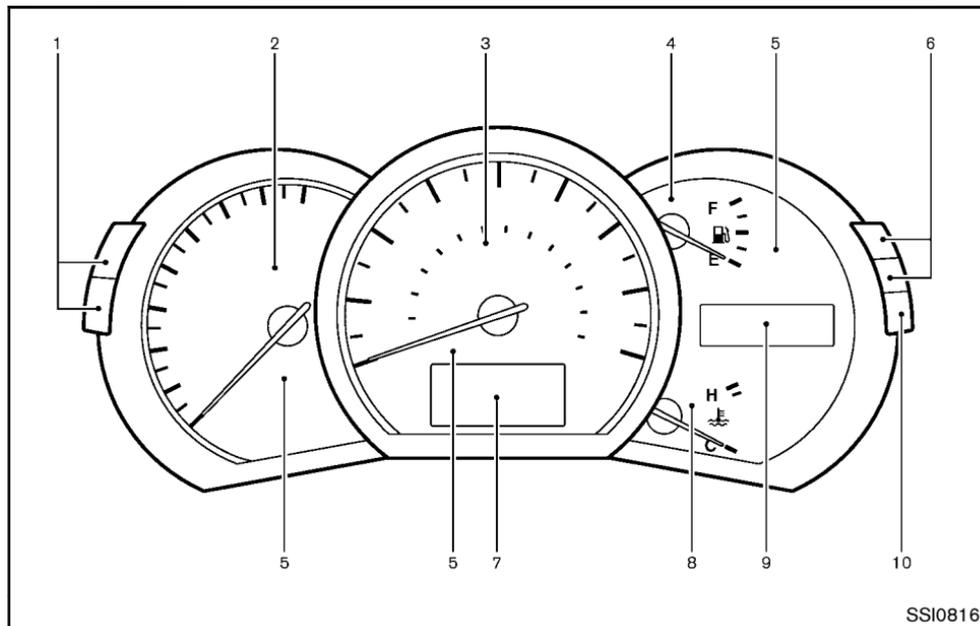
1. Instrument brightness control switch (P.2-39)
