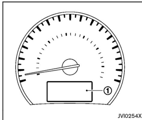
The dot matrix liquid crystal display  $\text{L1}$  is located in the speedometer, and it displays, the key operation information and other warnings and information.
