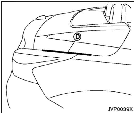
h. With two people, manually lift the storage lid by hand on the left and right side of the vehicle at lid edge **(D)**.
