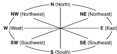
If the display reads “C”, calibrate the compass by driving the vehicle in 3 complete circles at less than 5 MPH (8 km/h). You can also calibrate the compass by driving your vehicle
