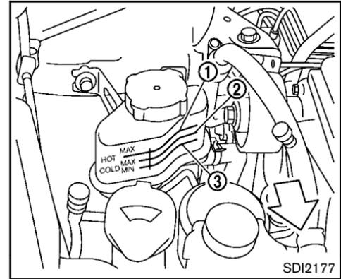
Check the fluid level in the reservoir.
