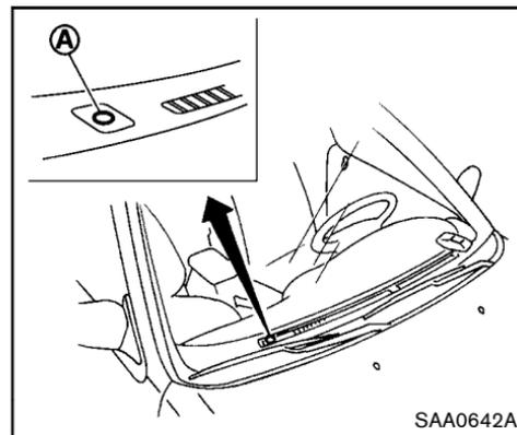
**Be sure not to put anything on top of the photo sensor ① located on the top of the instrument panel. The photo sensor controls the autolight; if it is covered, the photo sensor reacts as if it is dark and the headlights will illuminate.**
