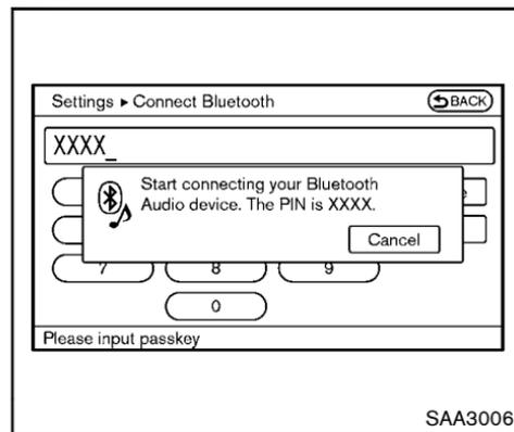
5. The standby message screen will appear. Operate the compatible Bluetooth® audio device. For the connecting procedure of the audio device, see the Bluetooth® audio instructions.
