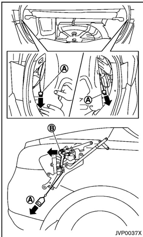
cables **(A)** in direction of arrow and release storage lid lock **(B)** .
