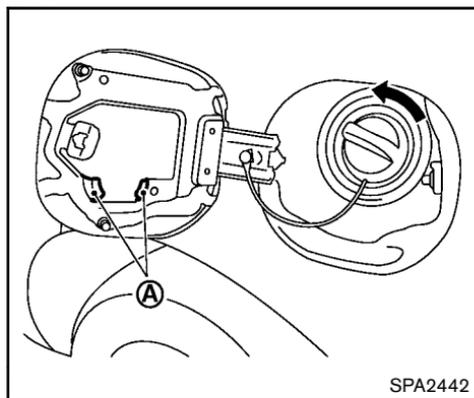
To remove the fuel-filler cap:
