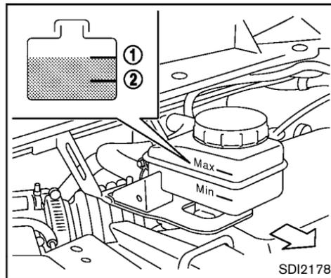
Check the fluid level in the reservoir. If the fluid is below the MIN line ② or the brake warning light comes on, add Genuine NISSAN Super Heavy Duty Brake Fluid or equivalent **DOT 3** fluid up to the MAX line ①. If fluid must be added frequently, the system should be checked by a NISSAN dealer.
