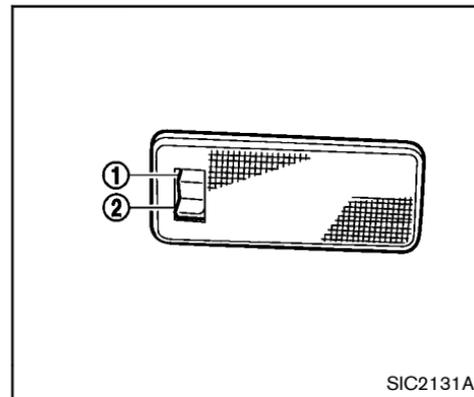
When the switch is in the ON position **1**, the light illuminates while the lift gate is opened. When the lift gate is closed, the light will turn off.
