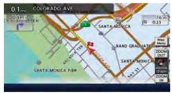
The current location map is displayed. An enlarged intersection view is automatically displayed when the vehicle approaches the guide point.
