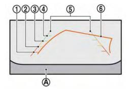
Guiding lines which indicate the vehicle width and distances to objects with reference to the bumper line (A) are displayed on the monitor.
