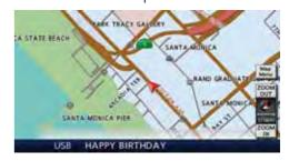
On the bottom of the map screen, the operating status of an audio/visual function is displayed at all times.
