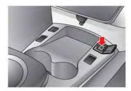
The auxiliary input jack is located on the center console.
