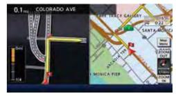
When approaching a guide point, the system automatically changes to the split screen and shows an enlarged view of the intersection on the left screen. To switch to the full screen mode while the enlarged intersection view is displayed, push the MAP button. Pushing the MAP button again displays the enlarged intersection view.
