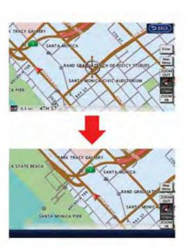
The basic map screen displays the current location (the position where the vehicle mark is located). Push the MAP button to display the current location on the map while on any screen.
