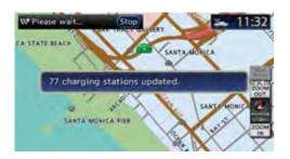
When connecting to the NISSAN CARWINGS Data Center, the system will periodically perform an automatic update of information for charging stations near your home. The system will also automatically update information for charging stations near the current vehicle location when the Li-ion battery charge is low. You can also manually update the charging stations around your current vehicle location at any time.
