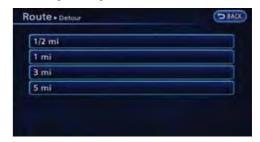
Touch a detour distance. After calculating the detour, the system displays the detour route on the map.
