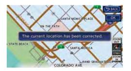
After adjusting the direction of the vehicle icon, touch [OK]. A message is displayed, and the adjusted vehicle location is stored.
