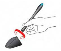
You can remove the antenna if necessary.
