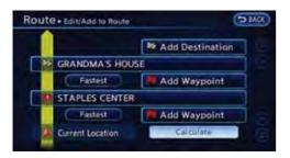
By touching [Calculate], the system will recalculate the routes. After the route search is completed, the display will automatically return to the current location map screen.
