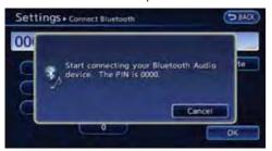
6. Touch [OK]. The standby message screen will appear. Operate the compatible Bluetooth® audio device. Please refer to the device's Owners Manual for the Bluetooth® audio connection instructions for your specific device. When the connection is completed, the screen will return to the Bluetooth® setup display.
