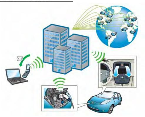
This vehicle incorporates a communication device that is called a TCU (Telematics Communication Unit). The communication connection between this unit and the NISSAN CARWINGS Data Center allows for various services.
