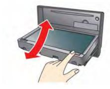
Open the monitor insert or ejecting a CD or an SD card.
