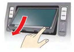
The angle of the monitor can be adjusted to select from 3 different preset angles. Once the angle of the monitor is selected and stored in the system, the selected angle is always set after performing the open/close operation of the monitor.
