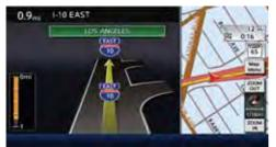
While driving on a freeway, when the vehicle is approximately 1 mile (approximately 2 km) from a junction, the system automatically switches to the split screen and displays an enlarged view of the junction on the left screen. After passing the junction, the system automatically returns to the full screen mode. To switch to the full screen mode while the enlarged junction view is displayed, push the **MAP** button. Pushing the **MAP** button again displays the enlarged junction view.
