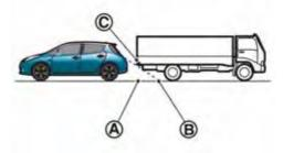
The position (C) is shown further than the position (B) in the display. However, the position (C) is actually at the same distance as the position (A). The vehicle may hit the object when backing up to the position (A) if
