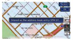
When a preferred location is displayed at the center of the map, confirm the address of the location and touch [OK]. A message is displayed, and the address of the location is stored in the Address Book.
