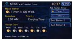
The air conditioner starts to operate at the time of day and day of the week specified in the settings. This pre cools or heats the passenger compartment before starting to drive. Electric power consumption from the Li-ion battery resulting from heater and air conditioner operation can be reduced because the temperature in the passenger room is adjusted before starting to drive.
