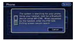
2. When a PIN code appears on the screen, operate the Bluetooth<sup>®</sup> compatible cellular phone to enter the PIN code.
