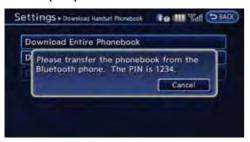
7. When a PIN code appears on the screen, operate the connected cellular phone to enter the PIN code. The downloading procedure of the cellular phone varies according to each cellular phone. See the cellular phone Owner's Manual for the details.
