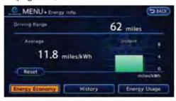
Estimated driving range and energy usage of various systems are displayed. Also, variation of the estimated driving distances between the climate control ON and OFF is displayed.
