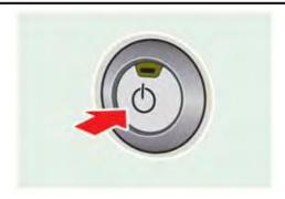
1. The system starts when the power switch is pushed to the "ACC" or "ON" position. The start-up screen is displayed.
