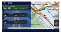
Depending on the setting, the system can constantly display the split screen and show the turn list on the left screen. When approaching a guide point, the left screen automatically switches to an enlarged view of the intersection. To switch to the full screen mode, push the **MAP** button. Pushing the **MAP** button again displays the turn list.
