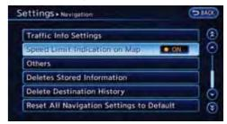
1. Touch [Speed Limit Indication on Map] to toggle the function between on and off. The indicator light illuminates when the speed limit display function is set to on.
