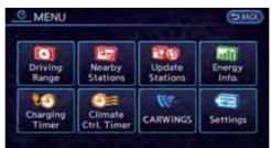
Push the <a>O</a> (Zero Emission menu) button to display the menu screen where several useful functions for electric vehicle driving can be set. Select a preferred menu and touch an item to be set.
