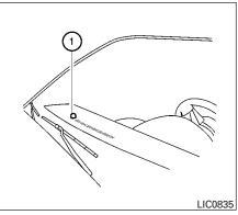
Be sure you do not put anything on top of the autolight sensor ① located on the top side of the instrument panel. The autolight sensor controls the autolight; if it is covered, the autolight sensor reacts as if it is dark out and the headlights will illuminate. If this occurs while parked with the engine off and the ignition switch placed in the ON position, your vehicle's battery could become discharged.
