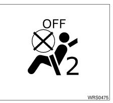
If the booster seat is installed in the front passenger seat, place the ignition switch in the ON position. The front passenger air bag status light may or may not illuminate, depending on the size of the child and the type of booster seat being used. See "Front passenger air bag and status light" later in this section.
