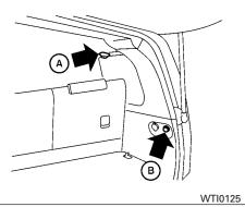
Cargo area ceiling tie-down hooks SECURING THE LOAD
