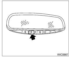
Using both hands, simultaneously press and hold both the HomeLink<sup>®</sup> button you want to program and the hand-held transmitter button.
