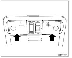
To turn the map lights on, press the switches. To turn them off, press the switches again.
