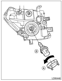
Removing the headlight bulb
