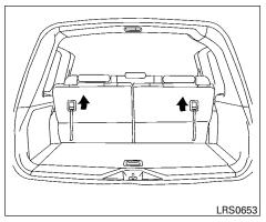
To return the 3rd row seats to a seating position, use the pull straps to raise each seatback. Pull back until the seatbacks latch into position. Make sure to properly raise each seatback to an upright and secured position.
