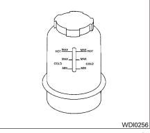
The fluid level should be checked using the HOT MAX range on the power steering fluid reservoir at fluid temperatures of  $122^{\circ} - 176^{\circ}F$  (50° - 80°C) or using the COLD MAX range on the power steering fluid reservoir at fluid temperatures of  $32^{\circ} - 86^{\circ}F$  (0° -  $30^{\circ}C$ ).
