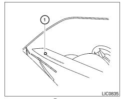
The sunload sensor ①, located on the top center of the instrument panel, helps the system maintain a constant temperature. Do not put anything on or around this sensor. Rear seat temperature and fan speed can be controlled from both the front seat overhead console controls or the rear seat controls (on back of center console).
