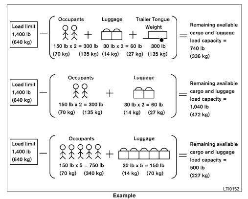
Steps for determining correct load limit
