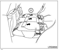
(3) There is a carpet panel flap on the back of each seat that can be folded toward the back of the vehicle.
