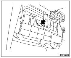
2. Lift upward on the retainer to release the filter cover and remove the filter cover.
