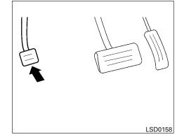
To engage: Firmly depress the parking brake.
