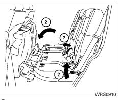
(2) Then lift up on the recline lever on the side of the outboard seats to fold the outboard seatbacks flat. To fold the center seatback flat, pull up on the strap on the edge of the center seat cushion and fold the seatback toward the front of the vehicle.
