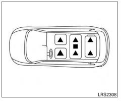
The illustration shows the seating positions equipped with head restraints/headrests. The first row head restraints are adjustable.
