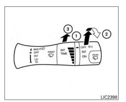
Push the switch forward ③ to operate the washer. Then the wiper will also operate several times.
