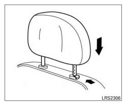
To lower, push and hold the lock knob and push the head restraint/headrest down.
