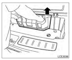
Remove the jack and tool kit cover by lifting up using the handles.
