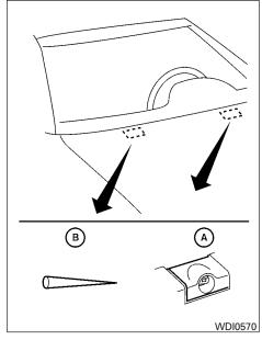
If you wax the surface of the hood, be careful not to let wax get into the windshield washer nozzle (A). This may cause clogging or improper windshield washer operation. If wax gets into the nozzle, remove it with a needle or small pin (B).
