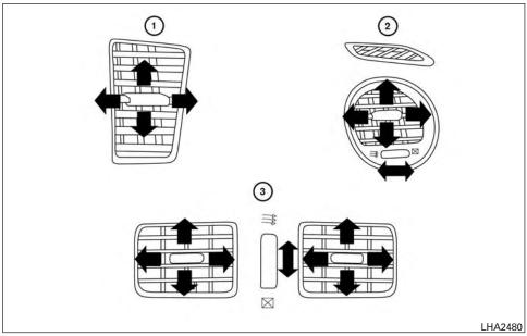
Adjust air flow direction for the center vents ①, driver's and passenger's side vents ②, and rear vents 3 by moving the vent slide and/or vent assemblies.
