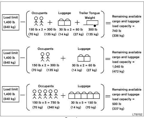
Steps for determining correct load limit
