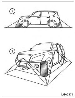
There are some areas where the system will not show objects. When in the front or rearview display, an object below the bumper or on the ground may not be viewed ①. When in the bird's-eye view, a tall object near the seam of the camera viewing areas will not appear in the monitor ②.
