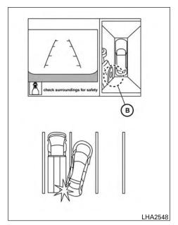
There may be a small distance visible between the vehicle and the object in the bird-eye view on the display (B).
