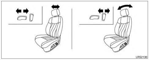
The reclining feature allows adjustment of the seatback for occupants of different sizes for added comfort and to help obtain proper seat belt fit. See "Precautions on seat belt usage" later in this section. Also, the seatback can be reclined to allow occupants to rest when the vehicle is stopped and the shift lever is in P (Park).
