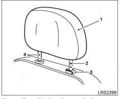
Non-adjustable head restraint/ headrest components
