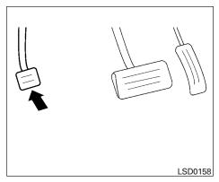
**To engage:** Firmly depress the parking brake.
