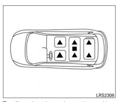
The illustration shows the seating positions equipped with head restraints/headrests. The third row head restraints are removable but not adiustable.
