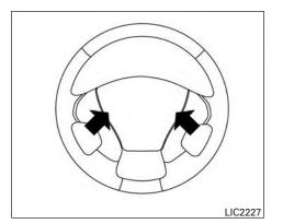
To sound the horn, push near the horn icon of the steering wheel.
