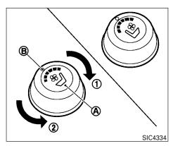
The climate controlled seat warms up or cools down the front seat by blowing warm or cool air from under the surface of the seat. The climate control switch is located on the center console.
