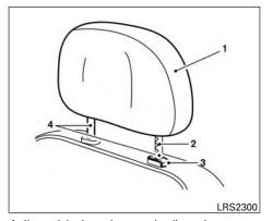
Adjustable head restraint/headrest components
