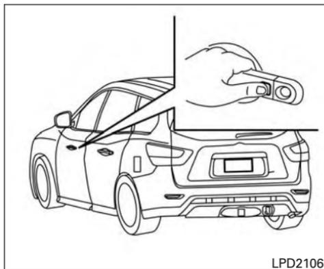
ing the door handle, push the door handle request switch to unlock the door.
