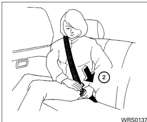
2. Slowly pull the seat belt out of the retractor and insert the tongue into the buckle ② until you hear and feel the latch engage.
