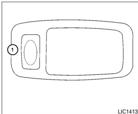
To turn on the personal lights, press and release the switch ①.
