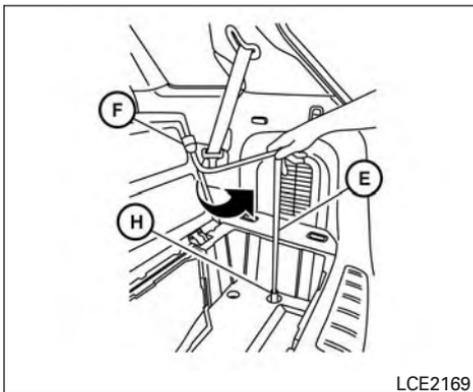
6. Insert the spare tire winch socket (H) to the lowering mechanism nut.
