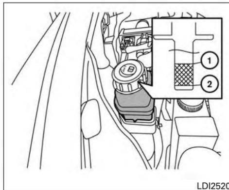
Check the fluid level in the reservoir.
