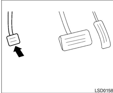
**To engage:** Firmly depress the parking brake.
