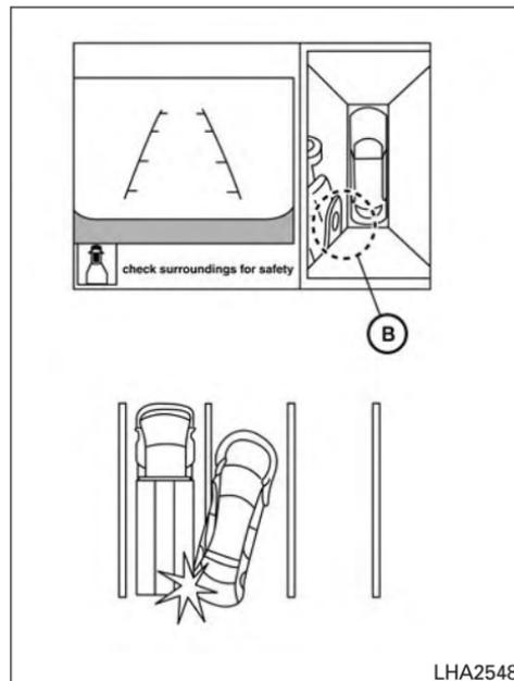
There may be a small distance visible between the vehicle and the object in the bird-eye view on the display (B).
