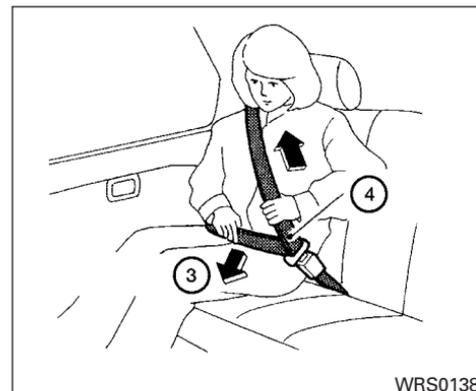
3. Position the lap belt portion **low and snug on the hips** ③ as shown.
