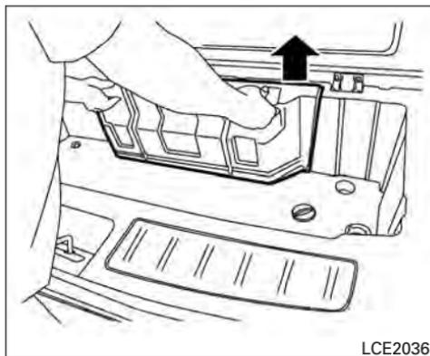
2. Remove the jack and tool kit cover by lifting up using the handles.
