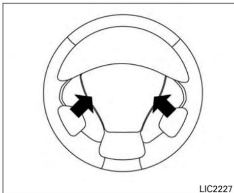
To sound the horn, push near the horn icon on the steering wheel.
