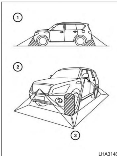
There are some areas where the system will not show objects and the system does not warn of moving objects. When in the front or rear view display, an object below the bumper or on the ground may not be viewed ①. When in the
