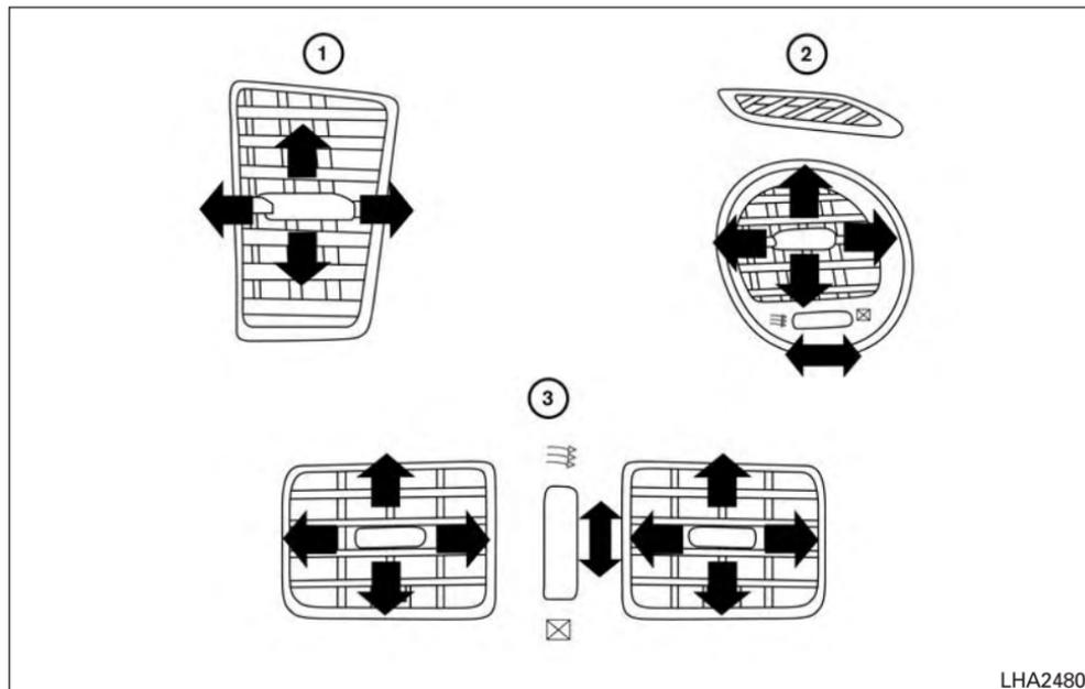
Adjust air flow direction for the center vents ①, driver's and passenger's side vents ②, and rear vents ③ by moving the vent slide and/or vent assemblies.
