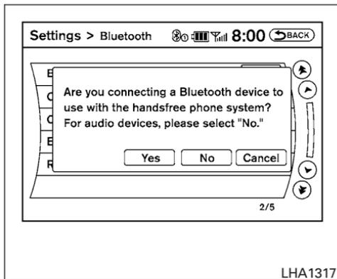
4. A screen will appear asking if you are connecting the device to use with the hands-free phone system. Select the “No” key.
