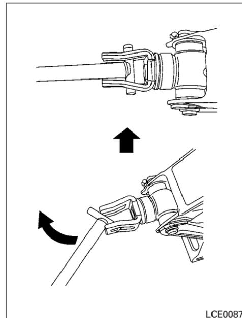
3. Install the assembled jack rod into the jack as shown.
