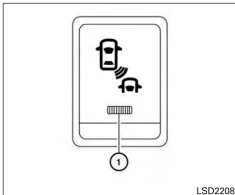
When the BSW and Rear Cross Traffic Alert (RCTA) system switch is turned off, the indicator ① on the switch is off. The indicator will also be off if the BSW/RCTA is deactivated.
