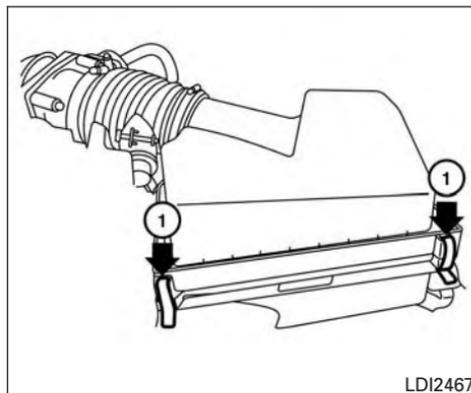
Clean and replace the air cleaner filter according to the maintenance log shown in the “NISSAN Service and Maintenance Guide”. When replacing the filter, wipe the inside of the air cleaner filter housing and the cover with a damp cloth.
