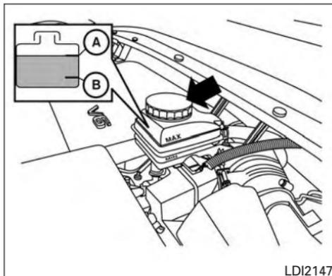
Check the fluid level in the reservoir. If the brake fluid is below the MIN line (B), the brake warning light will illuminate. Add brake fluid up to the MAX line (A). For additional information, refer to "Recommended fluids/lubricants and capacities" in the "Technical and consumer information" section of this manual for the recommended type of brake fluid.
