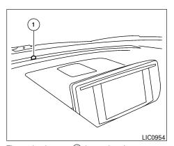
The sunload sensor ①, located on the top center of the instrument panel, helps the system maintain a constant temperature. Do not put anything on or around this sensor.
