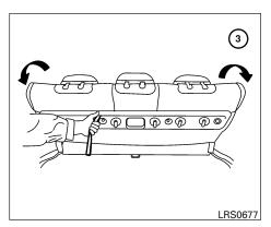
3. Pull back on the pull strap to release the back of the seat. Rotate the seatback toward the back of the vehicle.
