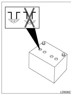
Check the fluid level in each cell. If it is necessary to add fluid, add only distilled water to bring the level up to the bottom of the filler opening. Do not overfill. Vehicles operated in high temperatures or under severe conditions require frequent checks of the battery fluid level.
