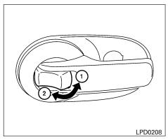
Inside lock for front doors LOCKING WITH INSIDE LOCK **KNOB**
