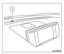
Be sure you do not put anything on top of the autolight sensor (1) located on top of the instrument panel. The autolight sensor controls the autolight; if it is covered, the autolight sensor reacts as if it is dark out and the headlights will illuminate. If this occurs while parked with the engine off and the key in the ON position, your vehicle's battery could become discharged.
