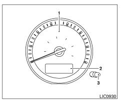
The twin trip odometer records the distance of individual trips.
