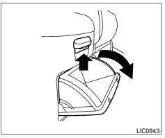
Pull up on the lever to access the front storage bin on the console box.
