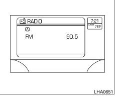
Any time audio information is shown on the main part of the screen, HVAC information will be displayed on the lower part of the screen. HVAC information will be shown even if "Audio" is selected to be displayed on the lower part of the screen.
