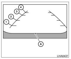
They are indicated as reference distances to objects. The lines and colors in the display indicate distances from the back bumper line (A) in the illustration.
