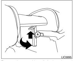
To store the tray table, pull the lever located beneath the tray table up (A) and gently lower the tray table to its original position.
