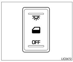
The lights on demand switch allows the driver to select one of three lighting modes for the interior lights. The lights on demand switch operates regardless of ignition switch position.
