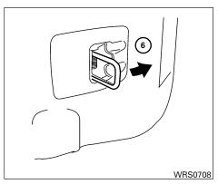
6. The rear seat anchors are spring loaded and can be folded into the side panels to maximize cargo space. The anchors are held in the folded position by the items in the cargo area. When the load is removed from the cargo area, the rear seat anchors automatically return to the unfolded position.
