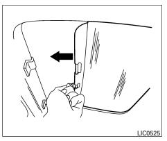
To close the SkyView roof sunshade, pull the tab to draw out the shade. Lock the shade in place by positioning the rod on the holder.
