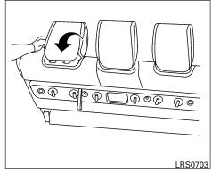
7. Reverse this process to return the bench seat to a seating position. Make sure to properly return the head restraints to the upright position, push the bench seat down into the floor, and pull back on the seatback until they latch into place.
