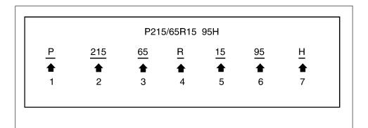
7. H: Tire speed rating. You should not drive the vehicle faster than the tire speed rating.
