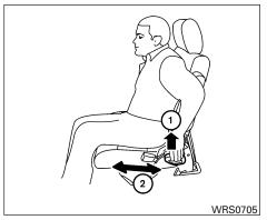
While seated, pull the lever 1 and hold it while you slide 2 the seat forward or backward to the desired position. Release the lever to lock the seat in position.
