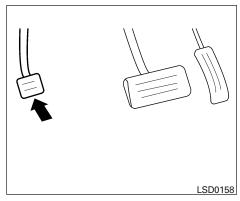
**To engage:** Firmly depress the parking brake.
