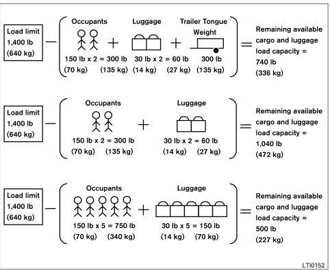
Steps for determining correct load limit
