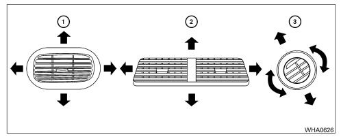
Adjust air flow direction for the driver and passenger side 1, center 2, and rear passenger 3 ventilators by moving the ventilator slide and/or ventilator assemblies.
