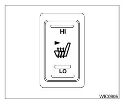
The front seats are warmed by built-in heaters (if so equipped). The switches are located at the sides of the seats.
