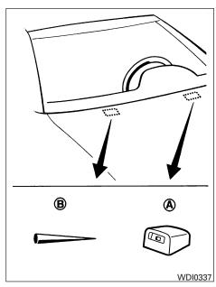
Be careful not to let anything get into the washer nozzle (a). This may cause clogging or improper windshield washer operation. If something gets into the nozzle, remove it with a needle or small pin (a).
