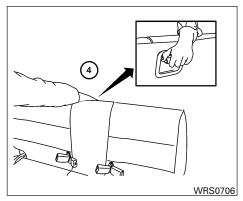
4. Pull up on the lever located on the back of the seat base. This will fold the seat base toward the back of the vehicle.
