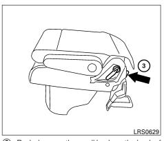
Push down on the small knob on the back of the seat to release the base of the seat.
