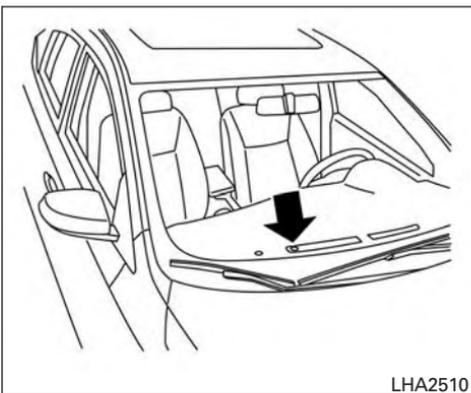
The sunload sensor (if so equipped), located on the top passenger's side of the instrument panel, helps the system maintain a constant temperature. Do not put anything on or around this sensor.
