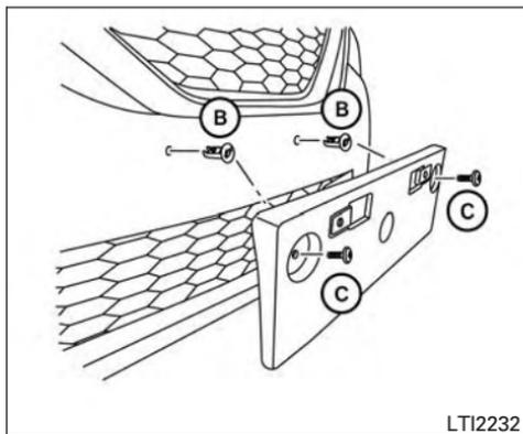
3. Insert two grommets (B) into the holes in the front bumper fascia.
