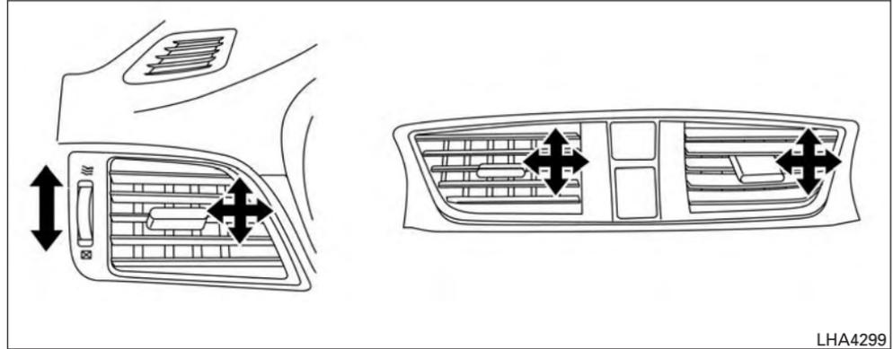
Adjust air flow direction by moving the vent slides.
