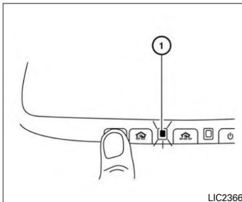
2. Using both hands, simultaneously press and hold the desired HomeLink® button and hand-held transmitter button. **DO NOT** release until the HomeLink® indicator light ① flashes slowly and then rapidly. When the indicator light flashes rapidly, both buttons may be released. (The rapid flashing indicates successful programming.)
