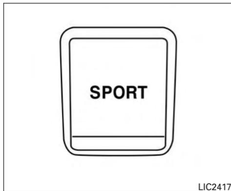
The SPORT mode switch adjusts the throttle sensitivity and transmission points to enhance performance. Push the SPORT switch on the instrument panel to activate. The SPORT mode indicator light (on the speedometer) will illuminate. The SPORT mode indicator light will remain lit while the mode is active.
