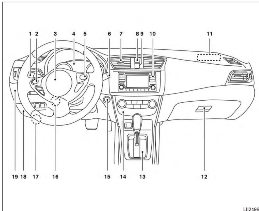
1. Headlight/fog light (if so equipped)/turn signal switch (P. 2-41)
