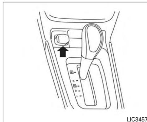
The power outlet is for powering electrical accessories such as cellular telephones. It is rated at 12 volt, 120W (10A) maximum.
