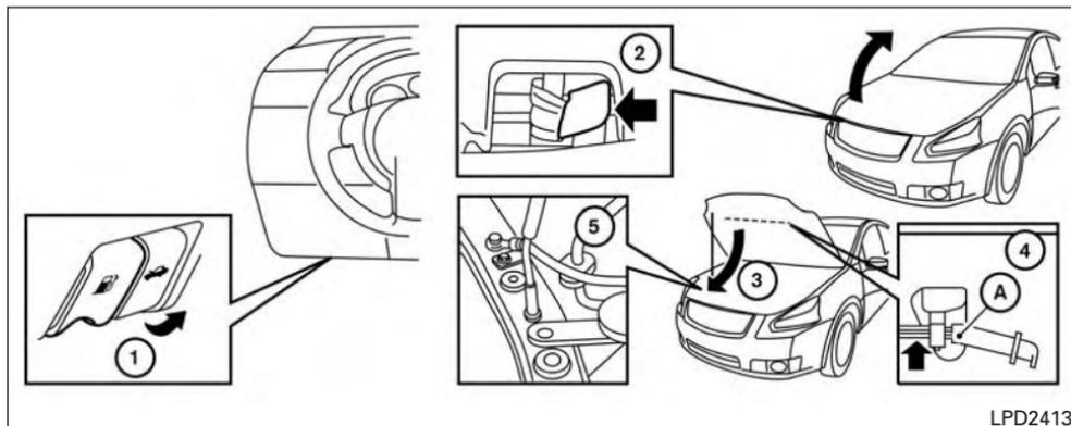
1. Pull the hood lock release handle (1) located below the instrument panel until the hood springs up slightly.
