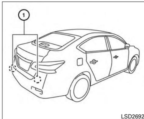
The BSW system uses radar sensors
