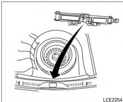
6. Install the jack in its storage area and tighten the jack strap.
