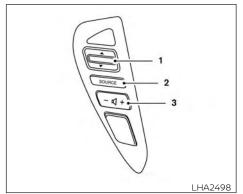
Type A (if so equipped) STEERING WHEEL SWITCH FOR **AUDIO CONTROL**
