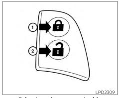
**Driver's and passenger's side**LOCKING WITH POWER DOOR
