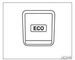
The ECO mode helps to enhance the fuel economy by controlling the throttle sensitivity and transmission points.
