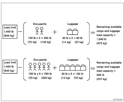
Steps for determining correct load limit
