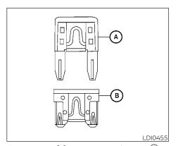
Two types of fuses are used. Type (A) is used in the fuse boxes in the engine compartment. Type **B** is used in the passenger compartment fuse box.
