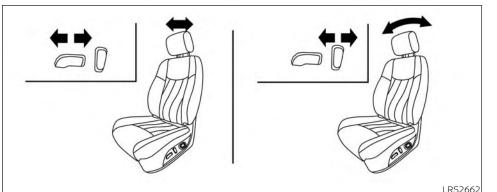
FRONT POWER SEAT ADJUSTMENT (if so equipped for driver's seat)
