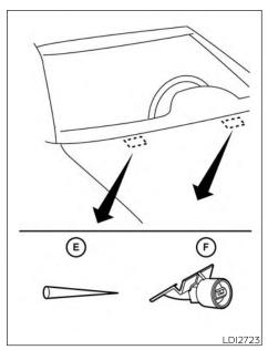
If you wax the surface of the hood, be careful not to let wax get into the washer nozzle (F). This may cause clogging or improper windshield-washer operation. If wax gets into the nozzle, remove it with a needle or small pin (E).
