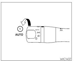
Autolight system (if so equipped) The autolight system allows the headlights to be set so they turn on and off automatically. The autolight system can:
