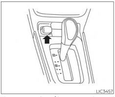
The power outlet is for powering electrical accessories such as cellular telephones. It is rated at 12 volt, 120W (10A) maximum.
