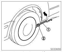
Removing wheel cover (if so equipped)
