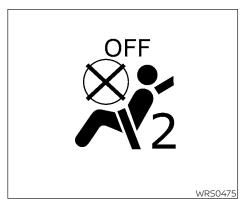
7. If the booster seat is installed in the front passenger seat, place the ignition switch in the ON position. The front passenger air bag status light 🌋 mav or may not illuminate, depending on the size of the child and the type of booster seat being used. For additional information, refer to "Front passenger air bag and status light" in this section.
