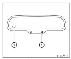
Type A (if so equipped) AUTOMATIC ANTI-GLARE REARVIEW MIRROR (if so equipped)
