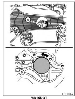
3. Place a large drain pan under the oil filter  $(\mathbf{B})$ .
