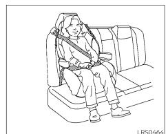
· Make sure the child's head will be properly supported by the booster seat or vehicle seat. The seatback must be at or above the center of the child's ears. For example, if a low back booster seat is chosen, the vehicle seatback must be at or above the center of the child's ears. If the seatback is lower than the center of the child's ears, a high back booster seat should be used
