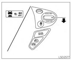
**To set cruising speed,** accelerate your vehicle to the desired speed, push the COAST/SET switch and release it. The ICC system set indicator (green), vehicle ahead detection indicator, set distance indicator and set vehicle speed indicator **®** will come on. Take your foot off the accelerator pedal. Your vehicle will maintain the set speed.
