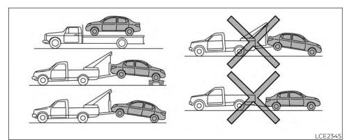
2WD models with Continuously Variable Transmission (CVT)
