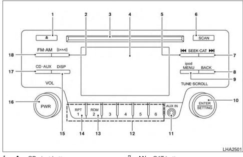
12. Station select (1 - 6) buttons 13. RDM button 14. RPT button 15. DISP button 16. VOL (volume) knob / PWR (power) button 17. CD-AUX button 18. FM-AM button
