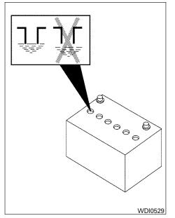
Check the fluid level in each cell. If it is necessary to add fluid, add only distilled water to bring the level up to the bottom of the filler opening. **Do not overfill.** Reinstall the vent caps. Vehicles operated in high temperatures or under severe conditions require frequent checks of the battery fluid level.
