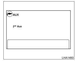
Press the AUX button to play a compatible device plugged into the AUX IN jack.
