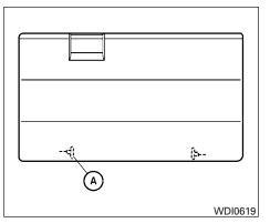
Remove the 2 lower glove box hinge pins
