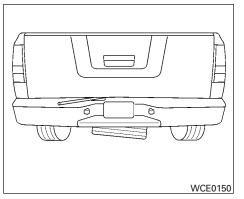
3. Assemble the two pieces of the jack rod. Find the oval-shaped opening above the middle of the license plate. Pass the T-shaped end of the jack rod through the opening and direct it toward the spare tire winch, located directly above the spare tire.
