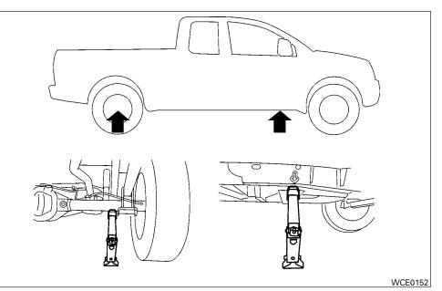
2. Place the jack directly under the jack-up point as illustrated so the top of the jack contacts the vehicle at the jack-up point. The jack-up points are indicated by stamped arrows on the side of the frame. The jack should be used on firm and level ground.
