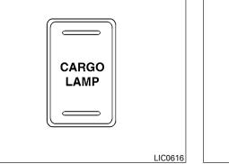
To turn on the cargo lamp, push the switch down to the ON position. The tailgate lights (if so equipped) will also illuminate when the cargo lamp switch is in the ON position.
