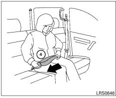
Loosen the belt by holding the tongue at a right angle to the belt, then pull on the belt. LRS0647
