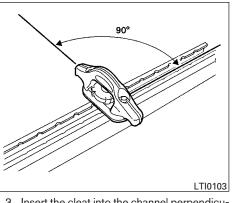
Insert the cleat into the channel perpendicular to the channel as shown. Then rotate the cleat clockwise 90° and slide it to the desired location.
