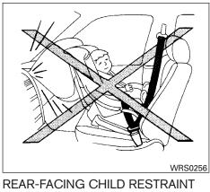
REAR-FACING CHILD RESTRAINT INSTALLATION USING THE SEAT BELTS
