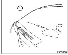
The sunload sensor ①, located on the top center of the instrument panel, helps the system maintain a constant temperature. Do not put anything on or around this sensor. The air conditioner system in your NISSAN vehicle is charged with a refrigerant designed with the environment in mind.
