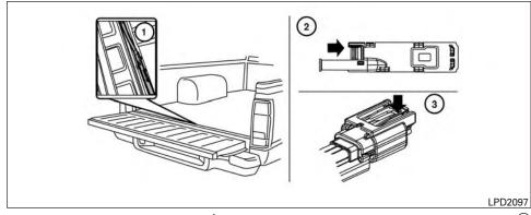
Disconnecting the rear camera (if so equipped)
