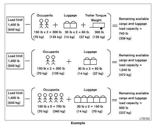
Steps for determining correct load limit
