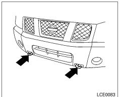
Hooks (if so equipped) VEHICLE RECOVERY (freeing a stuck vehicle)
