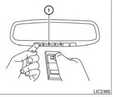
Using both hands, simultaneously press and hold the desired HomeLink<sup>®</sup> button and handheld transmitter button. DO NOT release until the HomeLink<sup>®</sup> indicator light (1) flashes slowly and then rapidly. When the indicator light flashes rapidly, both buttons may be released. (The rapid flashing indicates successful programming.)
