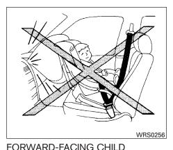
• NISSAN recommends that child restraints be installed in the rear seat. However, if you must install a forward facing child restraint in the front center bench seat, follow these instructions carefully.
