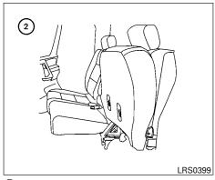
② Fold the bottom of the seat cushion toward the back of the vehicle until it locks in place.
