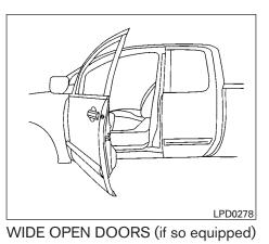
Do not open the Wide Open door to the full open position while the fuel-filler door is open; only open it as far as the first detent. Opening the door to the full open position may damage the fuel-filler door and Wide Open door.
