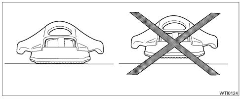
There should be no gap between the bottom of the cleat and the top of the channel. Tighten the center bolt hand tight (20-40 in-lbs).
