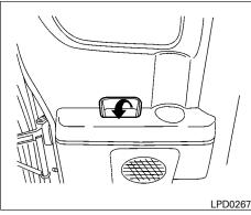
From the inside, pull the inside door handle toward you. The door will unlock automatically.
