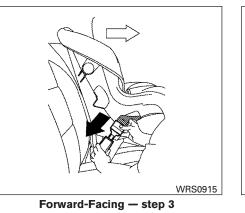
3. Route the seat belt tongue through the child restraint and insert it into the buckle until you hear and feel the latch engage.
