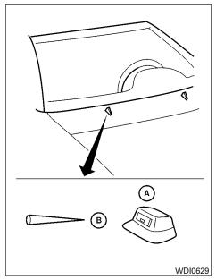
If you wax the surface of the hood, be careful not to let wax get into the windshield washer nozzle  $(\mathbf{A})$ . This may cause clogging or improper windshield washer operation. If wax gets into the nozzle, remove it with a needle or small pin  $(\mathbf{B})$ .
