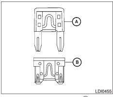
Two types of fuses are used. Type (A) is used in the fuse boxes in the engine compartment. Type (B) is used in the passenger compartment fuse box.
