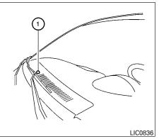
Be sure you do not put anything on top of the autolight sensor ① located on the top side of the instrument panel. The autolight sensor controls the autolight; if it is covered, the autolight sensor reacts as if it is dark out and the headlights will illuminate. If this occurs while parked with the engine off and the ignition switch placed in the ON position, your vehicle's battery could become discharged.
