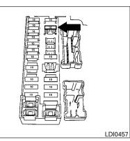
If a type A fuse is used to replace a type B fuse, the type A fuse will not be level with the fuse pocket as shown in the illustration. This will not affect the performance of the fuse. Make sure the fuse is installed in the fuse box securely.
