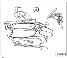
Folding the front passenger's seatback flat (if so equipped)
