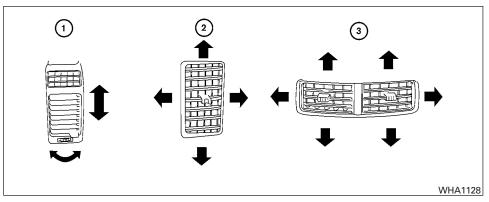
Adjust air flow direction for the driver's and passenger's side vents (1), center vents (2), and rear passengers' (if so equipped) vents (3) by moving the vent slide and/or vent assemblies.
