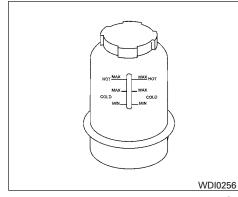
The fluid level should be checked using the HOT MAX range on the power steering fluid reservoir at fluid temperatures of  $122^{\circ} - 176^{\circ}F$  (50° - 80°C) or using the COLD MAX range on the power steering fluid reservoir at fluid temperatures of  $32^{\circ} - 86^{\circ}F$  (0° -  $30^{\circ}C$ ).
