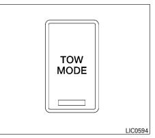
Tow mode should be used when pulling a heavy trailer or hauling a heavy load. Driving the vehicle in the tow mode with no trailer/load or light trailer/light load will not cause any damage. However, fuel economy may be reduced, and the transmission/engine driving characteristics may feel unusual.
