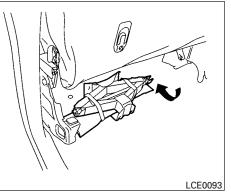
2. Unscrew and remove the jack and tool kit.
