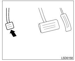
To engage: Firmly depress the parking brake.
