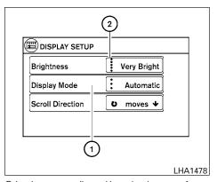
Other items are adjusted by selecting one of a set number of conditions. For example, the Display Mode can be set to "Automatic", "Day" or "Night". To adjust this type of item, touch the item ①. The item will cycle through the available settings and the red indicator lights to the left of the setting condition ② will come on or turn off accordingly.
