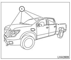
If dirt, rain or snow accumulates on any of the cameras (1), the Around View® Monitor may not display objects clearly. Clean the camera by wiping with a cloth dampened with a diluted mild cleaning agent and then wiping with a dry cloth.
