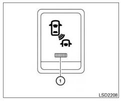
The warning systems switch is used to turn on and off the Blind Spot Warning (BSW) system that is activated using the settings menu on the vehicle information display.
