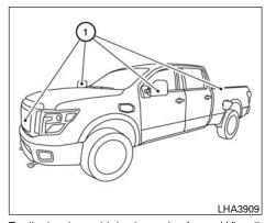
To display the multiple views, the Around View® Monitor system uses cameras located in the front grille, on the vehicle's outside mirrors and one on the tailgate (1).
