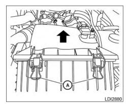
The air cleaner filter should not be cleaned and reused. Replace it according to the maintenance log shown in the "Titan Owner's Manual."
