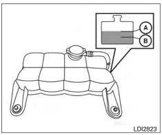
VK56VD engine CHECKING ENGINE COOLANT I FVFI
