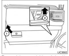
The extended storage switch is used when shipping the vehicle. It is located in the fuse panel inside the glove box. To reach it, open the glove box (1) on the instrument panel, then open the fuse panel cover (2).
