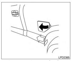
DIESEL EXHAUST FLUID (DEF) FILL CAP
