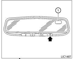
button for about 1 second when Press the -Nthe ignition switch is placed in the ON position to toggle the compass display 1 on or off. The display will indicate the direction of the vehicle's heading.
