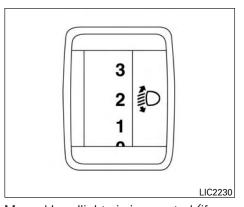
Manual headlight aiming control (if so equipped)
