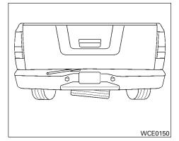
6. Assemble the pieces of the jack rod. Find the oval-shaped opening above the license plate, slightly to the left of the middle (driver's side). Pass the T-shaped end of the jack rod through the opening and direct it toward the spare tire winch, located directly above the spare tire.
