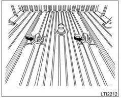
8. Rotate the safety chain anchor attachments 90° until the center of the anchor seats into place.
