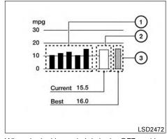
When the ignition switch is in the OFF position. ECO management display appears.
