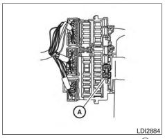
5. Remove the fuse with the fuse puller (A).
