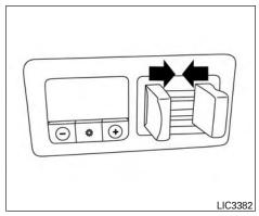
The TBCU on the instrument panel allows the driver to adjust the braking force applied to the trailer brakes.
