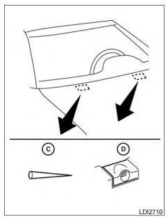
Be careful not to let anything get into the washer nozzle (D). This may cause clogging or improper windshield-washer operation. If something gets into the nozzle, remove it with a needle or small pin (C).
