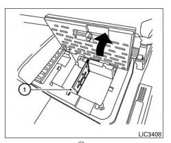
To adjust the divider (1), pull it straight up and reposition it to the desired location, sliding it straight down.
