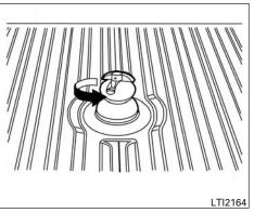
6. Rotate the handle 90° seat the handle back to the original resting position. If the handle does not seat fully, rotate the hitch ball until the handle drops into the original resting position.
