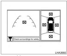
When the "[X]" icon is displayed on the screen, the camera image may be receiving temporary electronic disturbances from surrounding devices. This will not hinder normal driving operation but the system should be inspected by a NISSAN dealer if it occurs frequently.
