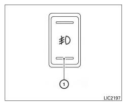
To turn the fog lights on, turn the headlight switch to the D position, then push the fog light switch (1) on.
