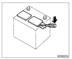
Remove the vent caps with a screwdriver as shown. Use a cloth to protect the battery case.
