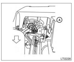
3. Locate the jumper harness connector under the lower portion of the instrument panel. The connector is taped to the wiring harness (A) as indicated.
