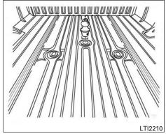
5. Position the ball bearings to the sides of the truck bed and Insert the gooseneck hitch ball into the center receiver tube of the truck bed.
