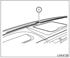
The sunload sensor ①, located on the top center of the instrument panel, helps the system maintain a constant temperature. Do not put anything on or around this sensor.
