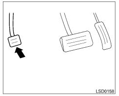
**To engage:** Firmly depress the parking brake.
