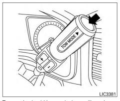
Tow mode should be used when pulling a heavy trailer or hauling a heavy load. Driving the vehicle in the tow mode with no trailer/load or light trailer/light load will not cause any damage. However, fuel economy may be reduced, and the transmission/engine driving characteristics may feel unusual.
