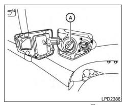
To remove the diesel fuel-filler cap f A:
