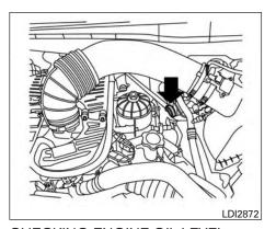
CHECKING ENGINE OIL LEVEL
