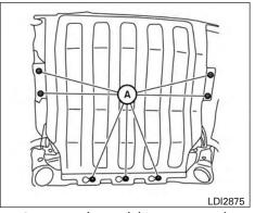
Skid plate (Type B) (if so equipped)
