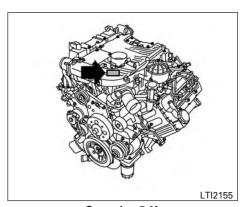
**Cummins 5.0L ENGINE SERIAL NUMBER**
