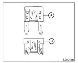
Two types of fuses are used. Type (a) and (b) are used in the fuse boxes in the engine compartment. Type (c) is used in the passenger compartment fuse box.
