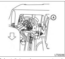
Locate the jumper harness connector under the lower portion of the instrument panel. The connector is taped to the wiring harness
