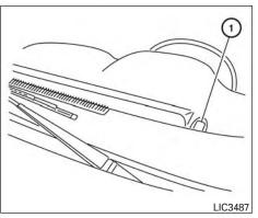
Be sure you do not put anything on top of the autolight sensor (1) located on the top side of the instrument panel. The autolight sensor controls the autolight; if it is covered, the autolight sensor reacts as if it is dark out and the headlights will illuminate. If this occurs while parked with the engine off and the ignition switch placed in the ON position, your vehicle's battery could become discharged.
