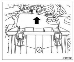
The dry paper type filter element may be cleaned and reused. Replace it according to the maintenance log shown in the "Titan Owner's Manual."
