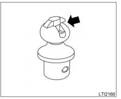
4. Lift the handle from the center of the hitch ball and rotate 90° from the resting position.
