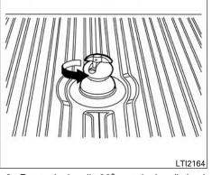
6. Rotate the handle 90° seat the handle back to the original resting position. If the handle does not seat fully, rotate the hitch ball until the handle drops into the original resting position.
