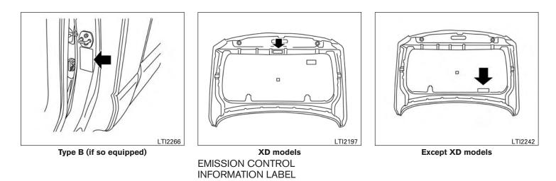
The emission control information label is attached to the underside of the hood as shown.
