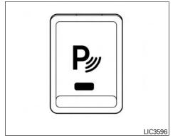
The parking sensor (sonar) system OFF switch on the instrument panel allows the driver to turn the parking sensor (sonar) system, Moving Object Detection (MOD), and Rear Cross Traffic Alert (RCTA) system on and off. To turn the systems on and off, the ignition switch must be in the ON position.
