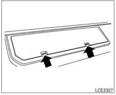
1. Open the passenger side rear door and remove the lid from the tool storage compartment.
