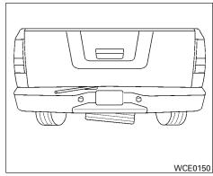
6. Assemble the pieces of the jack rod. Find the oval-shaped opening above the license plate, slightly to the left of the middle (driver's side). Pass the T-shaped end of the jack rod through the opening and direct it toward the spare tire winch, located directly above the spare tire.
