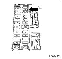
If a type (A) fuse is used to replace a type (B) fuse, the type (A) fuse will not be level with the fuse pocket as shown in the illustration. This will not affect the performance of the fuse. Make sure the fuse is installed in the fuse box securely.
