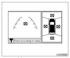
When the "[X]" icon is displayed on the screen, the camera image may be receiving temporary electronic disturbances from surrounding devices. This will not hinder normal driving operation but it is recommended that the system be inspected if it occurs frequently. It is recommend that you visit a NISSAN dealer for this service.
