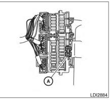
5. Remove the fuse with the fuse puller  $(\mathbf{A})$ .
