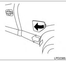
DIESEL EXHAUST FLUID (DEF) FILL CAP
