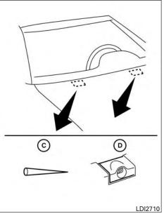
Be careful not to let anything get into the washer nozzle O. This may cause clogging or improper windshield-washer operation. If something gets into the nozzle, remove it with a needle or small pin C. If the brakes do not operate properly, have the brakes checked. It is recommended that you visit a NISSAN dealer for this service.
