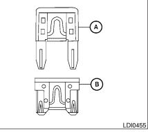
Two types of fuses are used. Type (A) and (B) are used in the fuse boxes in the engine compartment. Type (B) is used in the passenger compartment fuse box.
