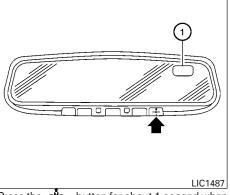
Press the - button for about 1 second when the ignition switch is placed in the ON position to toggle the compass display ① on or off. The display will indicate the direction of the vehicle's heading. N: North
