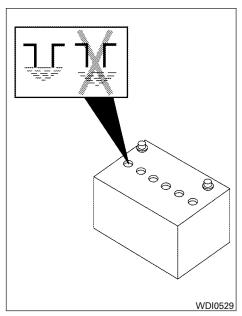
Check the fluid level in each cell. If it is necessary to add fluid, add only distilled water to bring the level up to the bottom of the filler opening. **Do not overfill.** Reinstall the vent caps.
