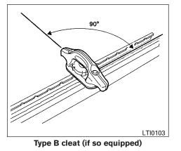
4. Position the cleat so the nubs on the bottom fully seat into the channel detents.
