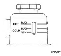
Check the power steering fluid level when the engine is stopped.
