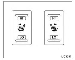
The rear seats are warmed by built-in heaters. The switches are located on the rear of the front center console and can be operated independently of each other.
