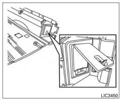
To open the bed liner storage bins on the tail gate end of the bed liner, lift the tab away from the truck bed, pull the lid up and away from the truck.
