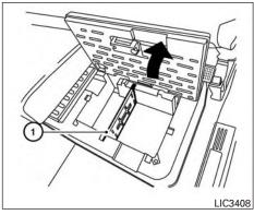
To adjust the divider (1), pull it straight up and reposition it to the desired location, sliding it straight down.
