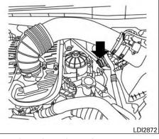
CHECKING ENGINE OIL LEVEL
