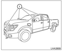
To display the multiple views, the Around View  $\mbox{$\mathbb{R}$}$  Monitor system uses cameras located in the front grille, on the vehicle's outside mirrors and one on the tailgate (1).
