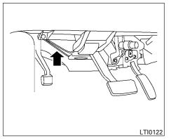
2. Apply the parking brake to access the jumper harness connector.
