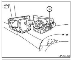
(-11°C), the DEF tank could freeze. In this condition, adding DEF will not change the gauge level and added DEF will not reach the pump, because it will sit on top of the frozen layer. Move the vehicle to a warm location to thaw the DEF completely for the gauge to read accurately and allow new DEF to reach the pump. If the tank is overfilled and freezes, it could be damaged, therefore do not overfill in sustained cold conditions below 12°F (-11°C).
