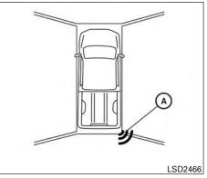
When the corner of the vehicle moves closer to an object, the corner sonar indicator (A) appears.
