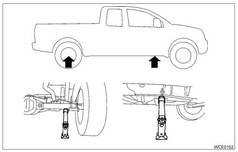
Always refer to the illustration for the correct placement and jack-up points for your specific vehicle model and jack type. Carefully read the caution label attached to the jack body and the following instructions.
