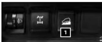
To deactivate Hill Descent Control, push the Hill Descent Control switch **1** to the OFF position.
