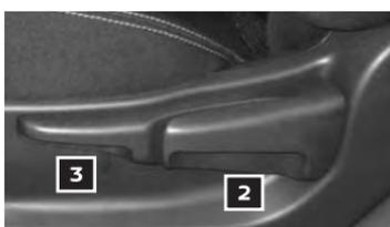
SEAT LIFTER (if so equipped for driver's seat)
