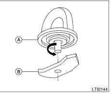
Assemble 4 hook loops (A) to 4 hook plates (B) by screwing the hook plate onto the hook (5 revolutions).
