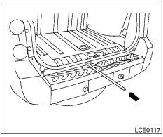
3. Find the oval-shaped opening above the middle of the bumper. Pass the T-shaped end of the jack rod through the opening and direct it toward the spare tire winch, located directly above the spare tire.
