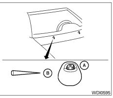
If you wax the surface of the hood, be careful not to let wax get into the windshield washer nozzle  $(\mathbf{A})$ . This may cause clogging or improper windshield washer operation. If wax gets into the nozzle, remove it with a needle or small pin  $(\mathbf{B})$ .
