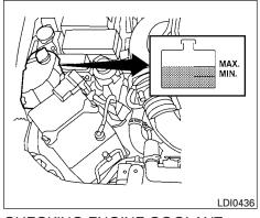
CHECKING ENGINE COOLANT LEVEL
