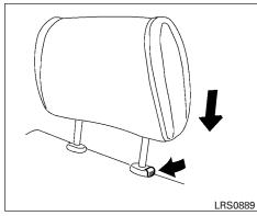
To lower, push and hold the lock knob and push the headrest down.
