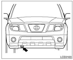
VEHICLE RECOVERY (freeing a stuck vehicle)
