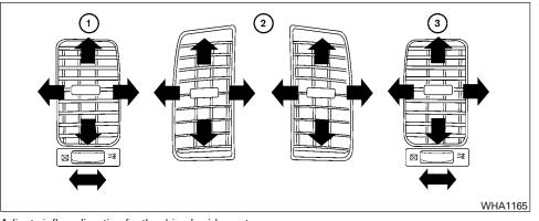
Adjust air flow direction for the driver's side vents (1), center vents (2), and passenger's side vents (3) by moving the vent slide and/or vent assemblies.
