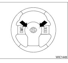
To sound the horn, push the area between the horn icons on the steering wheel.
