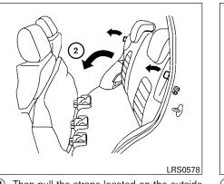
(2) Then pull the straps located on the outside edge of each seatback to fold the seatbacks forward.
