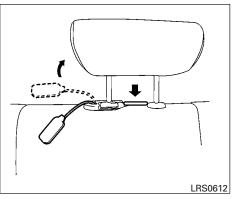
To return the seat belt comfort guide to the stowed position, route the comfort guide strap in the channel under the 2nd row driver's side seating position head restraint and attach the guide in the clip.
