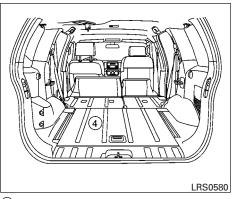
④ To return the bench seats to a seating position, reverse this process. Raise the seatbacks to an upright position. Make sure to hold the seat belts above the seat cushion, then push the seat cushion down into place.
