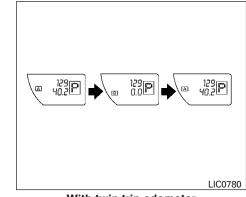
With twin trip odometer Changing the display:
