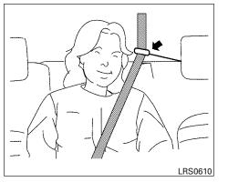
Insert the shoulder belt into the back of the comfort guide so that the seat belt lays flat in the guide. Be sure that the comfort guide routes the seat belt properly over the center of your shoulder and across your chest. The belt should be away from your face and neck, but not falling off of your shoulder.
