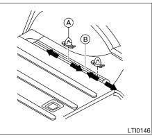
Insert (at any position) 2 channel tie-down hooks (A) into the channel opening (B) of each channel and slide to the desired position.
