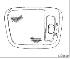
The cargo light on the overhead trim has a threeposition switch. To operate, push the switch to the desired position.
