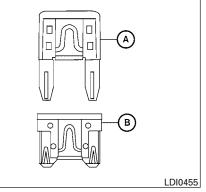
Two types of fuses are used. Type (A) is used in the fuse boxes in the engine compartment. Type (B) is used in the passenger compartment fuse box.
