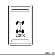
The Electronic Locking Rear Differential (E-Lock) system can help provide added traction if the vehicle is stuck or becoming stuck.
