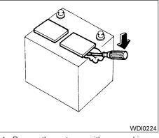
1. Remove the vent caps with a screwdriver as shown. Use a cloth to protect the battery case.
