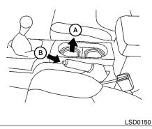
To engage: Pull the parking brake lever up (A).
