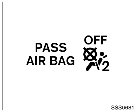
Front passenger air bag status light
