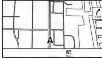
When route guidance starts, the small turn arrow and the distance to the next guide point are displayed in the upper right corner of the map screen. This arrow indicates the turning direction at the next guide point (corner or intersection). When approaching a guide point, enlarged intersection view is displayed. Also, there may be cases where next street names are announced.
