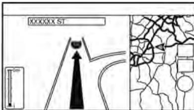
While driving on a freeway, when the vehicle is approximately 1 mile (approximately 2 km) from a junction, the system automatically switches to the split screen and displays an enlarged view of the junction on the left screen. After the vehicle passes the junction, the system automatically returns to the full screen mode. To switch to the full map screen while the enlarged junction view is displayed, push **<MAP>**.
