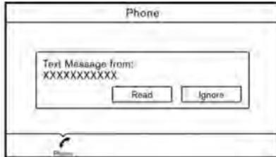
When the cellular phone connected to the vehicle receives a text message, a notification will appear on the vehicle information display and on the touch screen display with a tone.
