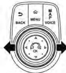
Slide the slide switch leftward to scroll to the previous page. Slide the slide switch rightward to scroll to the next page.
