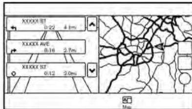
When [Turn List] in the view settings menu is turned on, a turn list can be displayed on the left side of the screen. To switch to the full map screen, push **<MAP>**.
