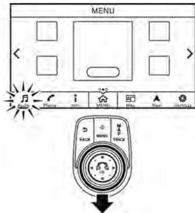
Sliding the slide switch backwards will enable the center dial operation of the Launch Bar. Slide the switch forward to return to operate Shortcuts with the center dial.
