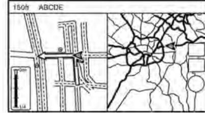
When approaching a guide point, the system automatically changes to the split screen and shows an enlarged view of the intersection on the left screen. To switch to the full map screen while the enlarged intersection view is displayed, push **<MAP>**. The distance to the guide point and the name of the next street to drive on are displayed on the top of the screen.
