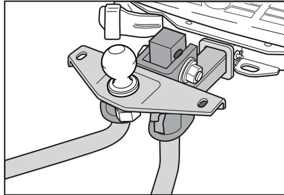
**Clamp-On Bumper Hitch** – This temporary hitch clamps onto the bumper assembly.
